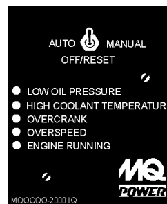
Figure 34. MPEC Engine Running Status LED (OFF)
