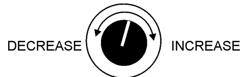
Figure 10. Voltage Regulator Control Knob
