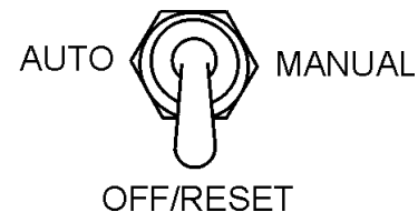
Figure 64. Off/Manual Auto Switch (OFF)
