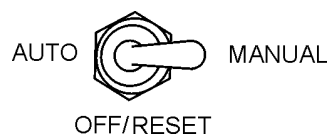
Figure 58. Engine Controller Switch (Manual)
