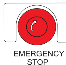
Figure 58 . Emergency Stop Button
