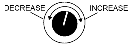
Figure 24. Voltage Regulator Knob 3Ø 200/208V (50/60 Hz), 1Ø 115/120V (50/60Hz) Output Terminal Lug Voltages
