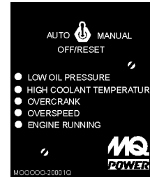
Figure 23. Microprocessor Engine Controller (MPEC)
