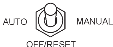
Figure 65. Off/Manual Auto Switch (Off)
