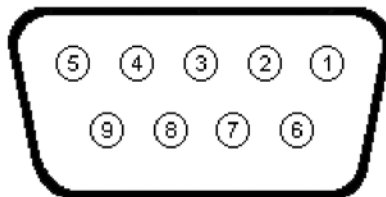
Figure 4-5. MODBUS Communication Port Terminal Positions
