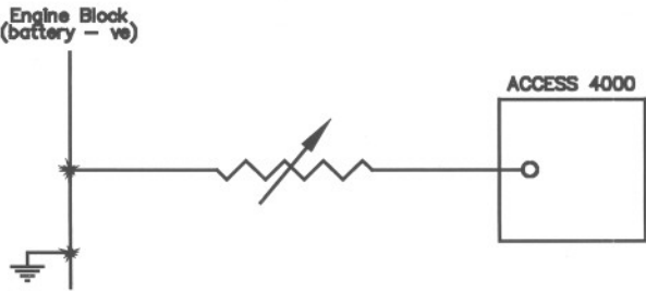
Figure 2.4 - Typical DC Sender Input Wiring
