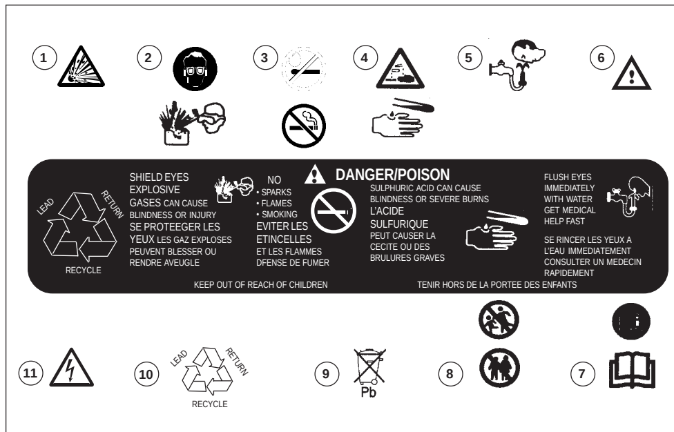
Fig. 1—Typical Battery Labelling
