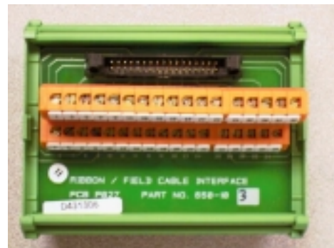
Ribbon/Field Cable Interface
