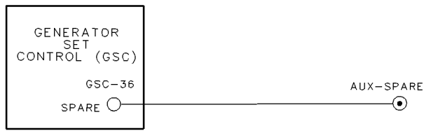
Illustration 51 System Schematic For Spare Output When used as a high/low logic circuit.
