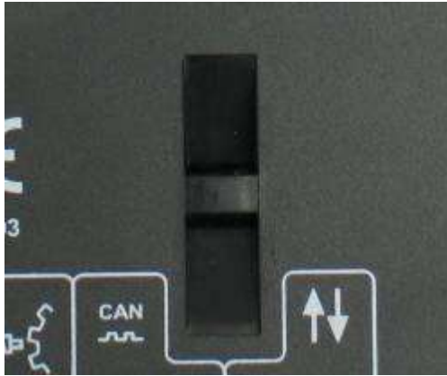
Cable Tie Fixing Point
