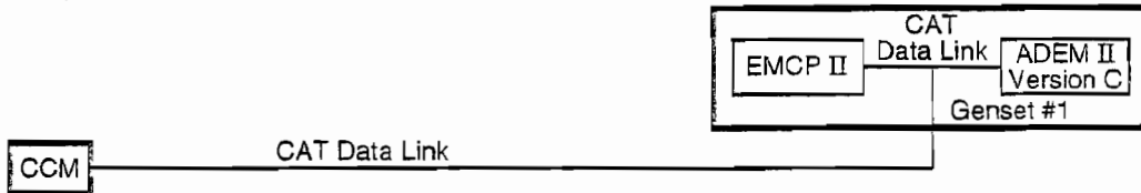
Example 6 - 3500B EUI Genset (Version C ECM) with EMCP II (Basic Model)
