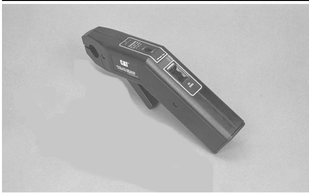
Illustration 16 g00538441 8T - 0900 AC/DC Clamp-On Ammeter
