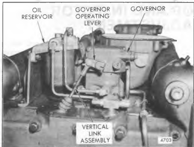
Fig. 4 - Hydraulic Governor Mounting and Linkage (Former with Vertical Link)
