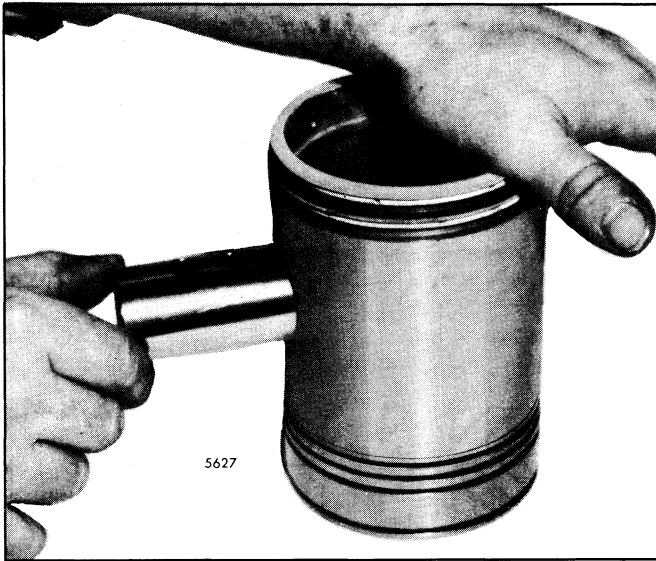
Fig. 15 - Installing Piston Pin
