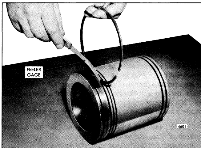
Fig. 8 - Measuring Piston Ring Side Clearance
