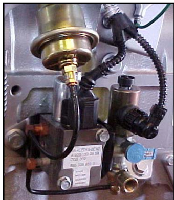
Engine mounted solenoid valve turbo brake configuration
