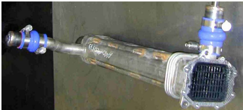
Figure 3 - EGR cooler ports: plugged
