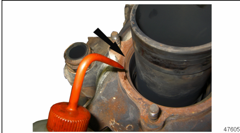
Figure 6 Applying Penetrating Oil to Matrix Lip
