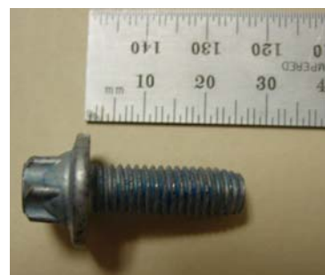
Self tapping bolt for CTV Cover plate 2 (P/N: 000000001140)
