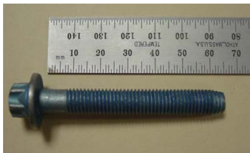
Self tapping bolt with use of CTV solenoid 2 (P/N: 000000001535)
