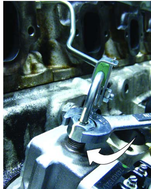
Figure 5 Turning Fuel Line Nut 120 Degrees at Unit Pump End
