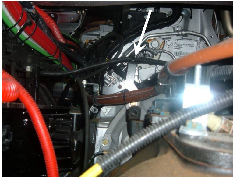
Figure 12 - Block Heater Cable Fastener on Left Side of Cylinder Head
