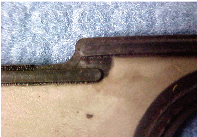
Figure 15. Open vent head gasket.
