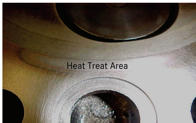
Figure 10. Head with heat treated combustion area and recessed grommet area.
