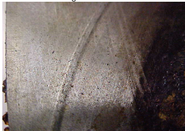
Figure 11. Raised section of combustion sealing area.
