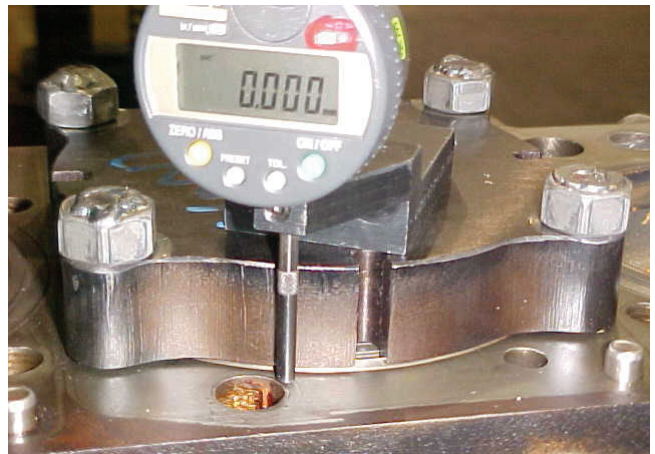
Figure 24. Measuring cylinder liner protrusion.
