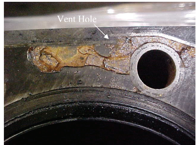
Figure 2. Head gasket vent hole witness marks.
