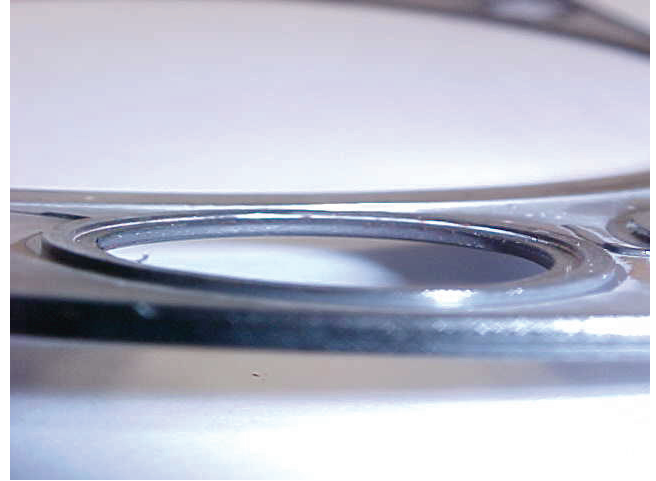
Figure 16. Gasket with flat grommet.
