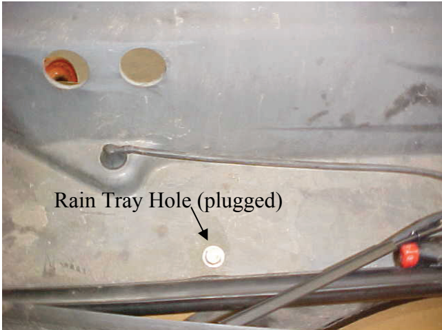
Figure 3. Plugging the rain tray drain hole may reduce water draining on top of engine.
