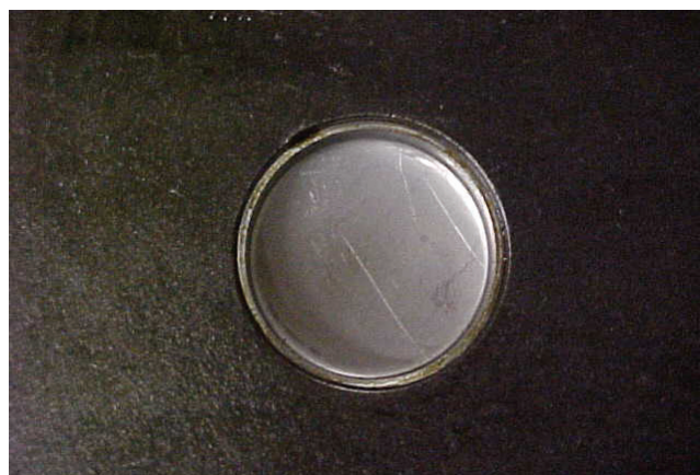
Figure 12. Cylinder head with cup plug.
