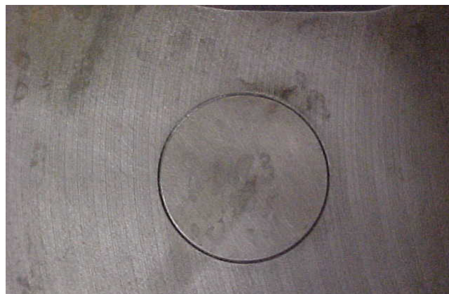
Figure 13. Cylinder head with solid plug.
