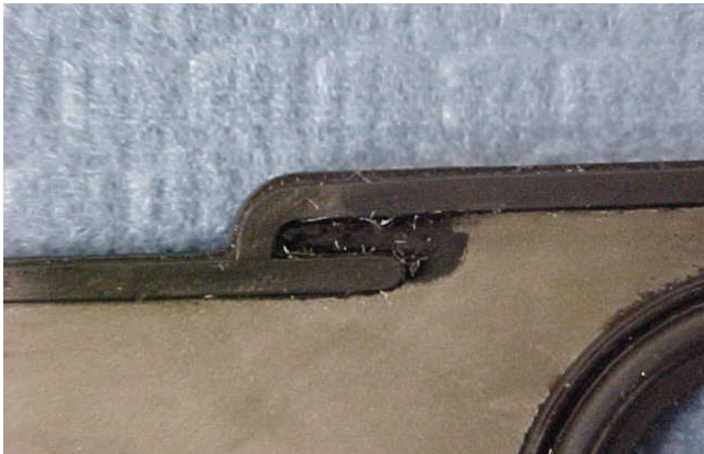
Figure 14. Closed vent head gasket.
