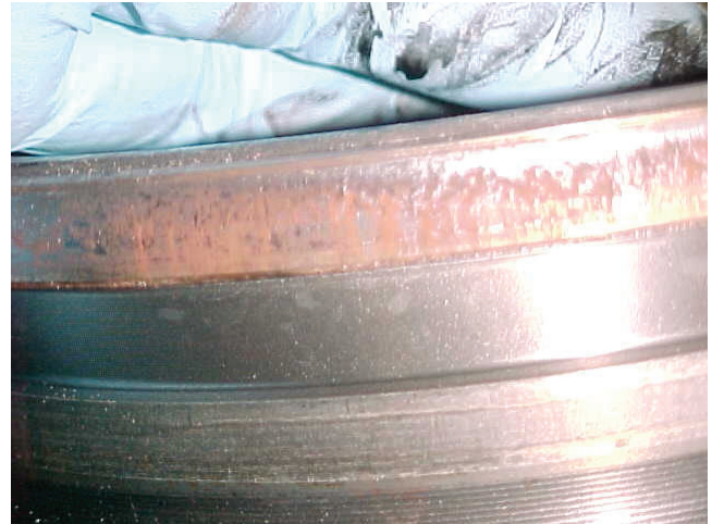
Figure 5. Fretting around cylinder liner from high mileage.
