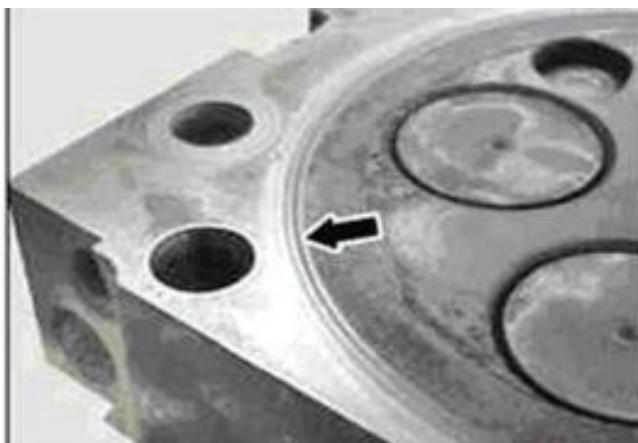
Figure 9. Cylinder head with no recess around oil and coolant grommet areas.
