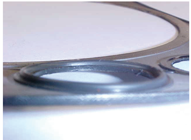
Figure 17. Gasket with raised grommet.
