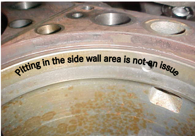
Figure 22. Sidewall pitting is not critical.
