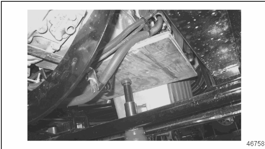
Figure 1 Floor Jack Engine Support by Shallow Portion of Oil Pan
