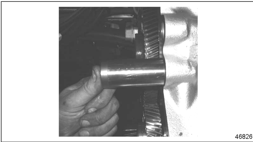
Figure 6 Tool Properly Seated Against Block
