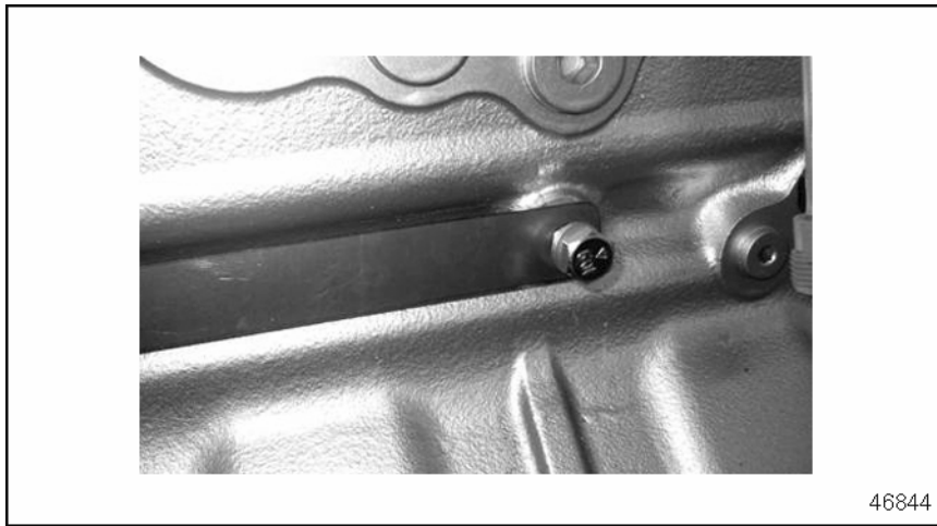
Figure 3 Install the M10 Bolt to Secure Bracket to Block
