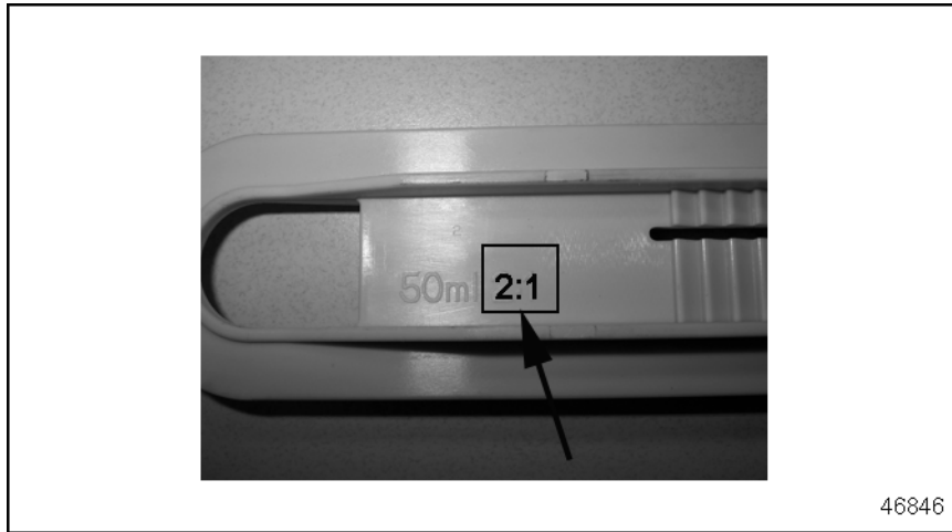
Figure 5 Mixture Ratio listed on Trigger Gun Ram
