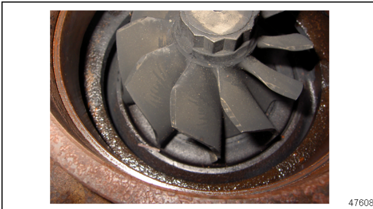
Figure 9 Checking Turbine Blades for wear
