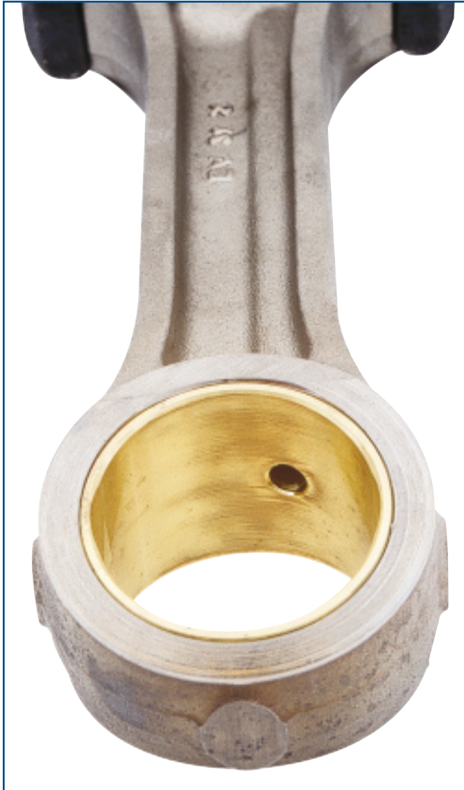
Connecting rod bushing machining marks are still visible indicating minimal wear.
