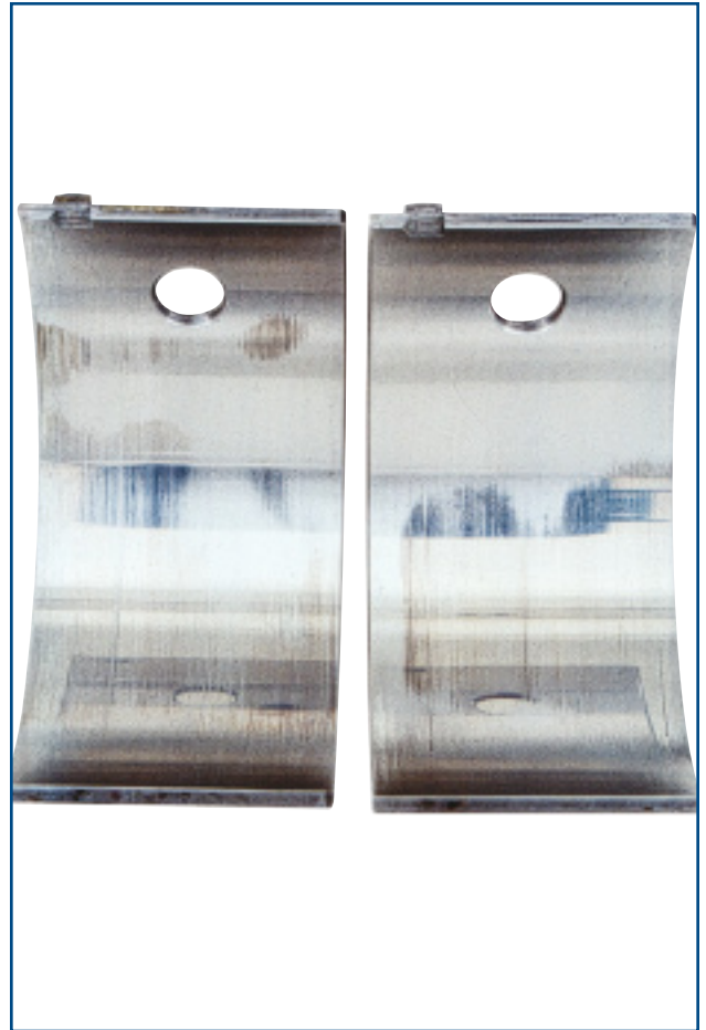
Cam bearings show minor polishing.
