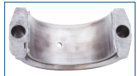
Rod bearings show only minor overlay wear.
