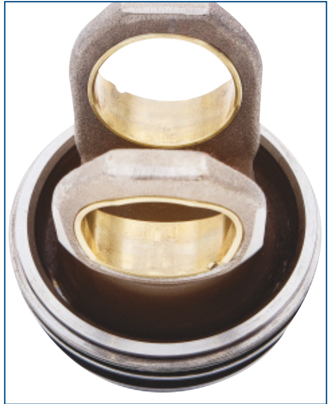
Piston bushings only show typical polishing.
