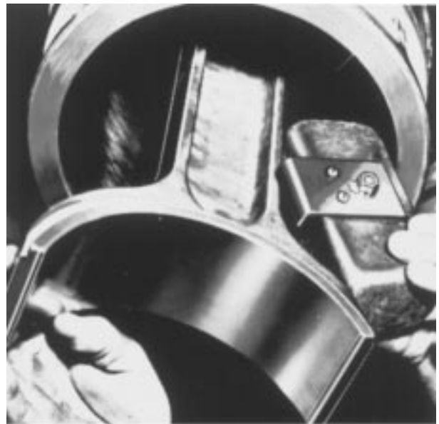
9080908 Locator - Crab Bolt - 645 Engines (used to center Crab Bolts)
