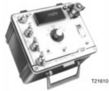
9322571 Ohmmeter - Digital Low Resistance - Kit includes the following: 9322574 Ohmmeter - Range 0 to 19.99 ohms in 5 ranges - 0 to 1.999 milliohms lowest range - four digit display 9322575 Battery Charger - With Batteries 9322576 Leads - Six foot Helical Spring Point 9322577 Batteries - For Ohmmeter (used in 9322574 meter only) (Battery Charger not shown)
