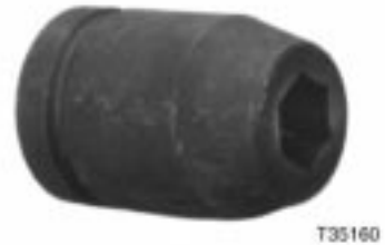
40034178 Socket - Used for removing bolts on aluminum end Bell Unit of Traction Motor Armatures
