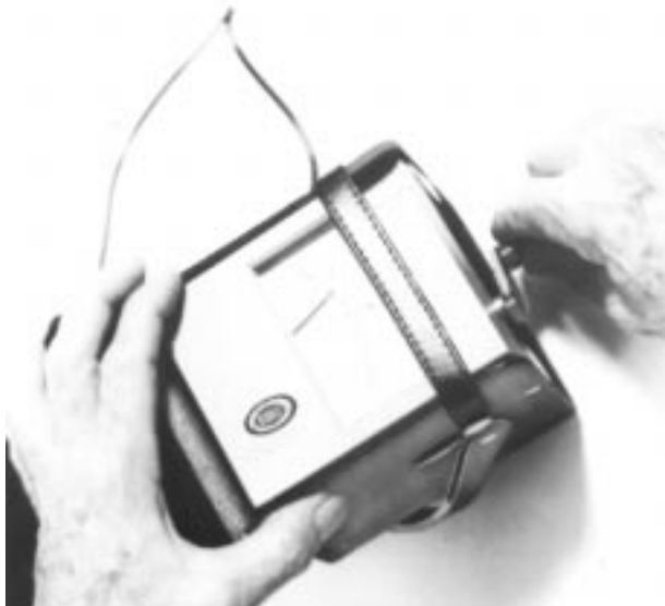
8174880 Tester - Insulation Resistance - Megger 0-2000 megohms, 1000 volts - 0-1000 megohms, 500 volts - 0-500 megohms, 250 volts - Generator Type 8174878 Lead - Heavy Duty - Pair 12 ft. long 8174879 Case - Carrying
