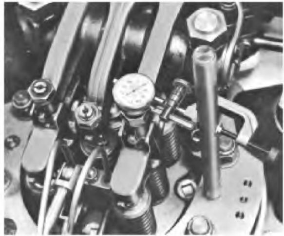
Fig. 7-20 - Timing Exhaust Valves
