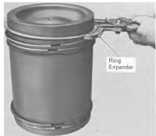
Fig. 3-8 - Removing Piston Rings
