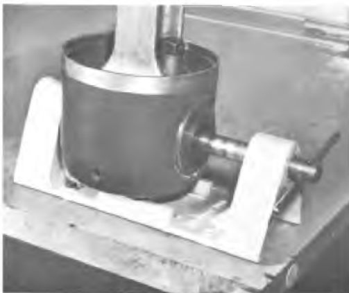
Fig. 5-16 - Carrier In Holding Fixture
