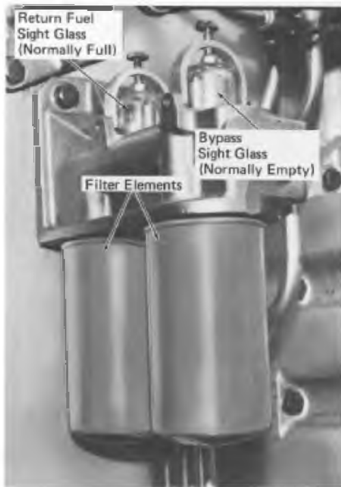
Fig. 11-13 - Fuel Filter
