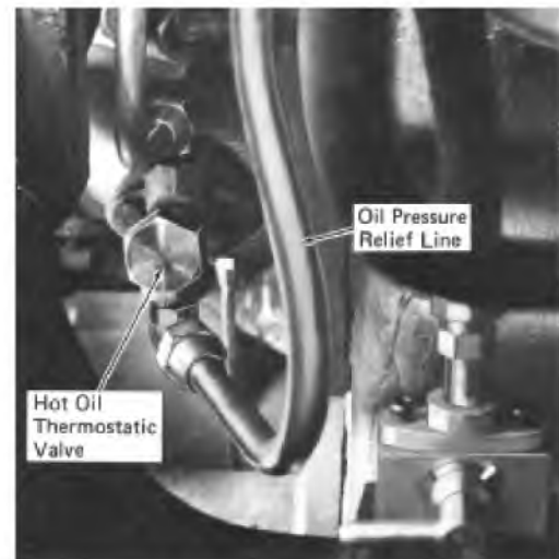
Fig. 13-10 -Hot Oil Shutdown Installation
