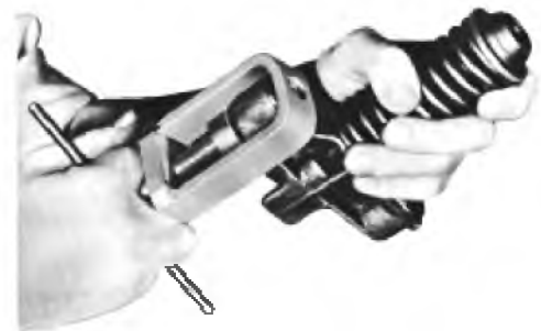
Fig. 2-28 - Installing Lash Adjuster
