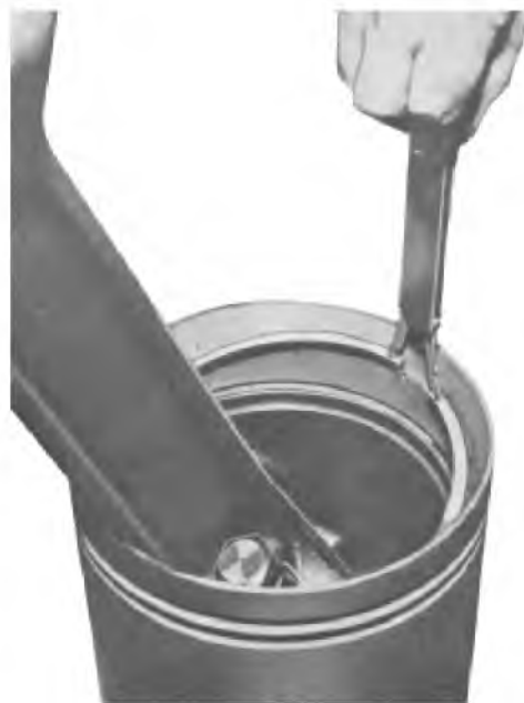
Fig. 5-17 - Installing Piston Snap Ring
