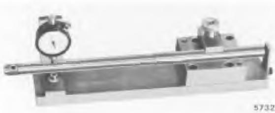
Fig. 2-12 - Tapered Pilot Checking Fixture
