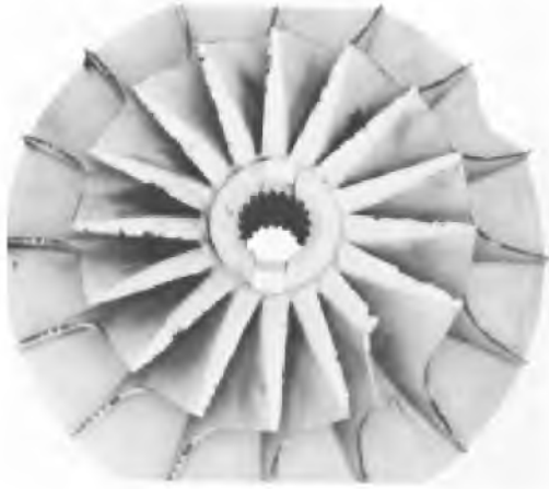
Fig. 15-16 - Impeller Damaged By Foreign Material
