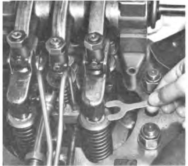
Fig. 15-9 - Checking Lash Adjuster To Valve Clearance
