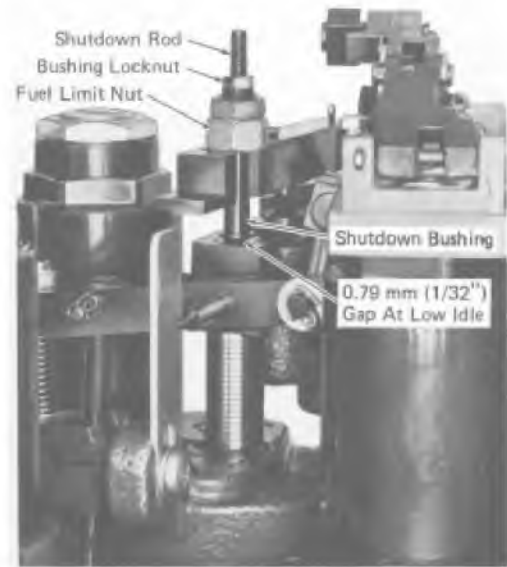
Fig. 12-7 - Shutdown Adjustment Location
