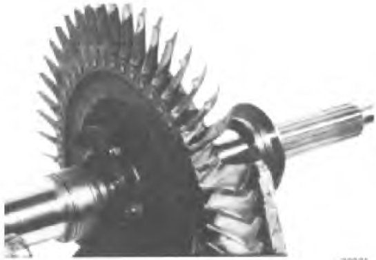
Fig. 15-18 - Stretched Blades That Have Rubbed The Shroud
