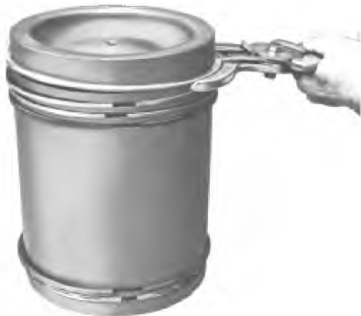
Fig. 5-14 - Installation Of Top Compression Ring
