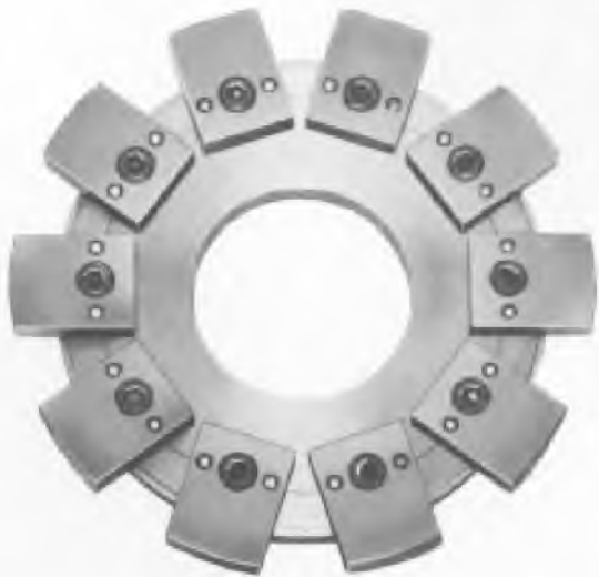
Fig. 3-11 - Piston Ring Groove Gauge
