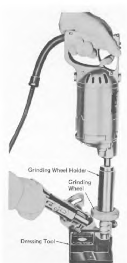
Fig. 2-10 - Dressing Valve Seat Grinding Wheel
