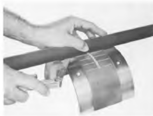
Fig. 3-15 - Checking Rod Upper Bearing Shell
