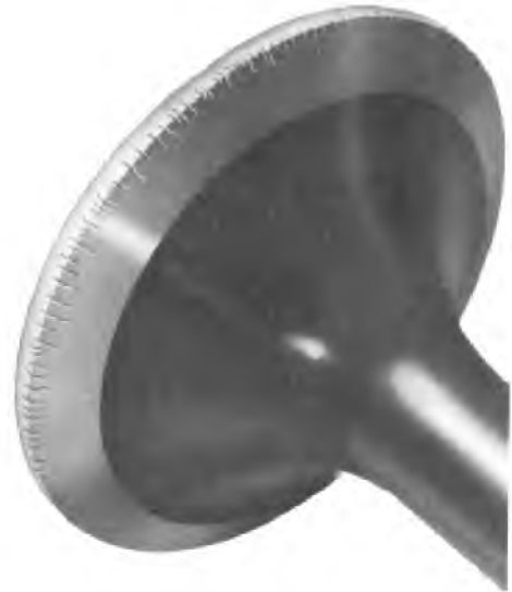
Fig. 2-19 - Face And Ring Defects
