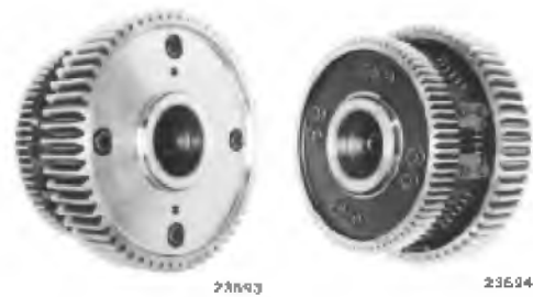
Fig. 7-3 - Spring Drive Gear Assembly
