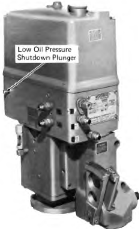
Fig. 13-1 - Low Oil Pressure Shutdown Plunger
