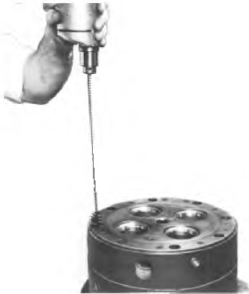
Fig. 2-4 - Cleaning Stud Holes
