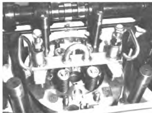
Fig. 5-6 - Cylinder Head Removing Fixture
