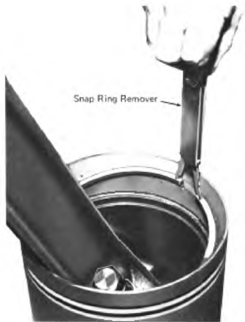
Fig. 3-6 - Removing Piston Snap Ring
