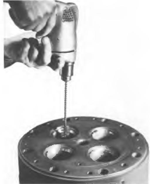
Fig. 2-5 - Cleaning Valve Guides
