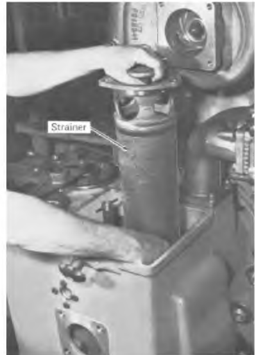
Fig. 9-8 - Scavenging Oil Pump Strainer
