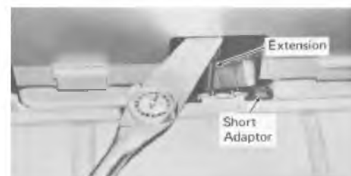
CENTER BOLT TIGHTENING
