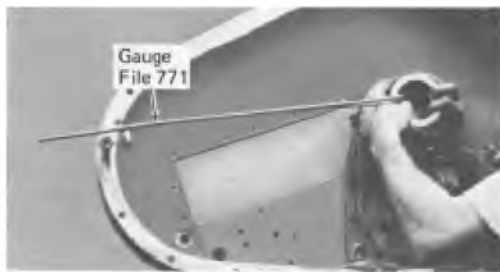
Fig. 7-10 - Camshaft Drive Housing Alignment
