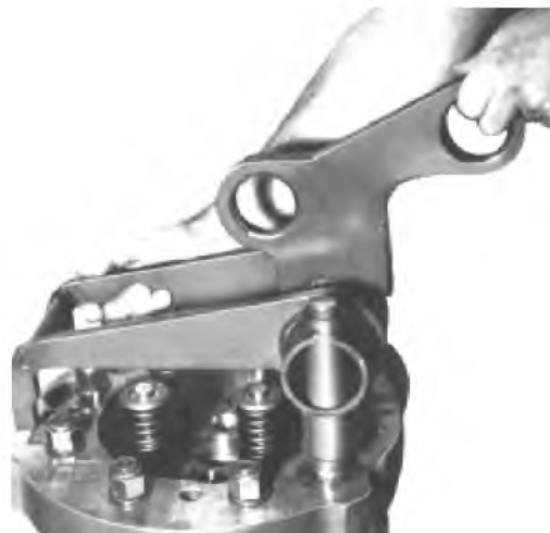
Fig. 5-10 - Lifting Clamp Application
