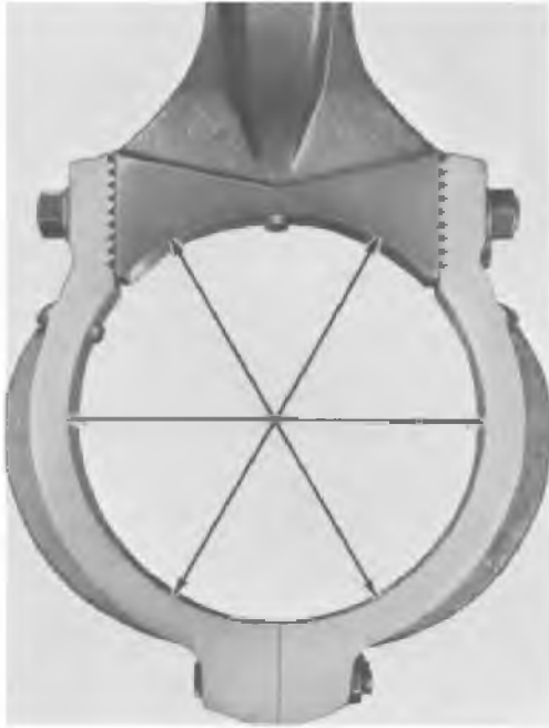
Fig. 3-14 - Checking Fork Rod Bore
