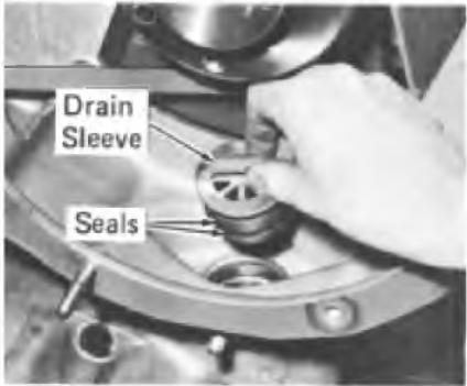
Fig. 13-8 - Overspeed Trip Housing Drain Sleeves
