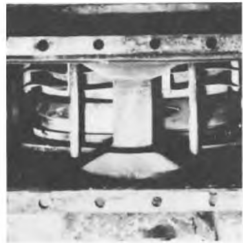
Fig. 15-20 - View Down The Exhaust Stack Of A Warped Diffuser And Damage From Broken Blades
