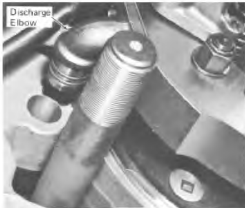
Fig. 5-34 - Water Discharge Elbow Alignment
