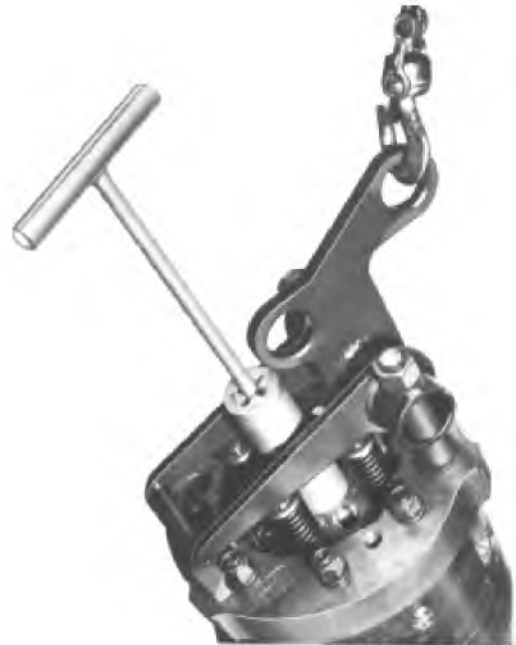
Fig. 5-32 - Power Assembly Installation With Lifting Clamp And Hoist
