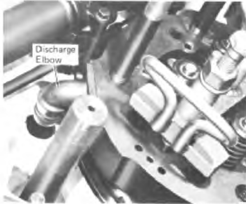
Fig. 5-22 - Water Discharge Elbow Alignment
