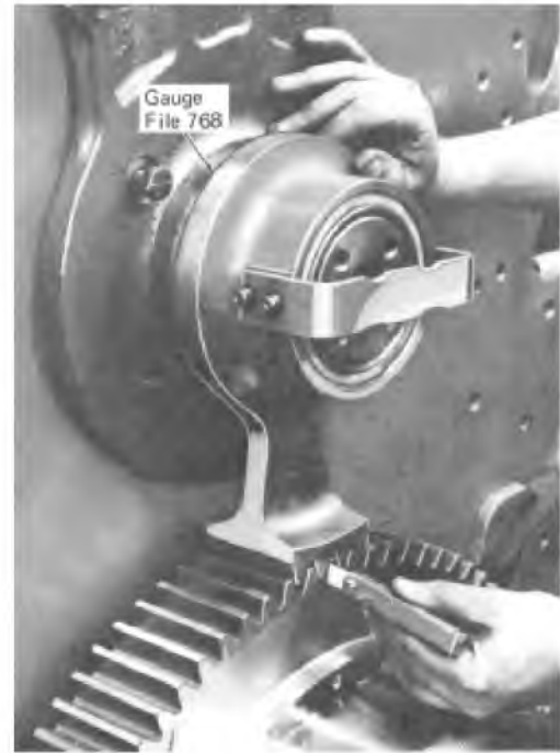
Fig. 7-6 - Checking No. 1 Idler Gear To Crankshaft Gear Backlash
