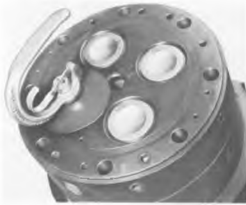
Fig. 2-22 - Testing Valve Seat Seal
