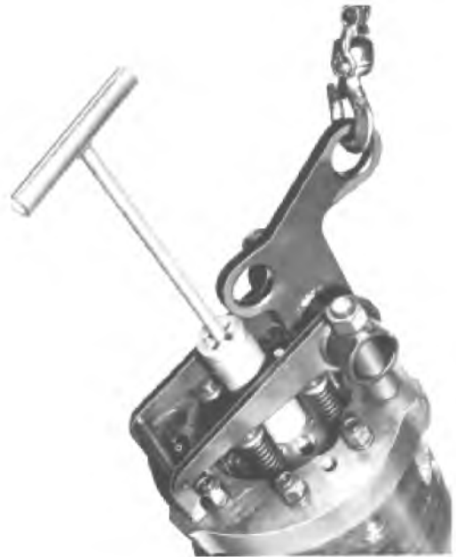
Fig. 5-13 - Power Assembly Removal 22115 With Lifting Clamp And Hoist
