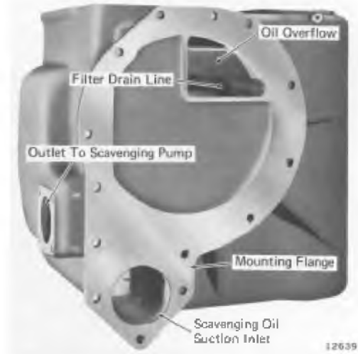
Fig. 9-6 - Oil Strainer Housing
