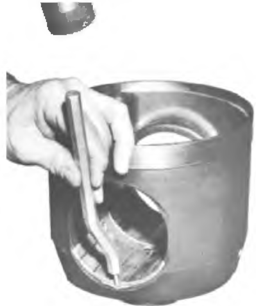
Fig. 5-15 -- Piston Pin Bearing Insert Installation
