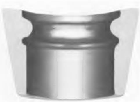
Fig. 2-20 - Valve Spring Seat Lock
