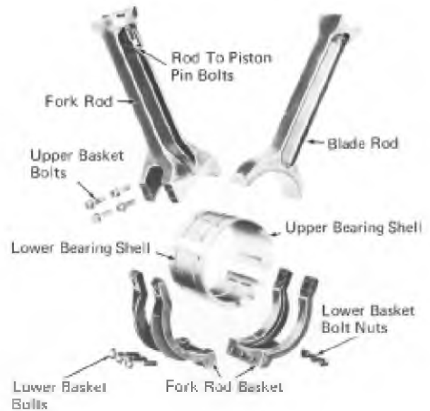
Fig. 3-12 -"Connecting" Rods, Bearing Shells, And Basket
