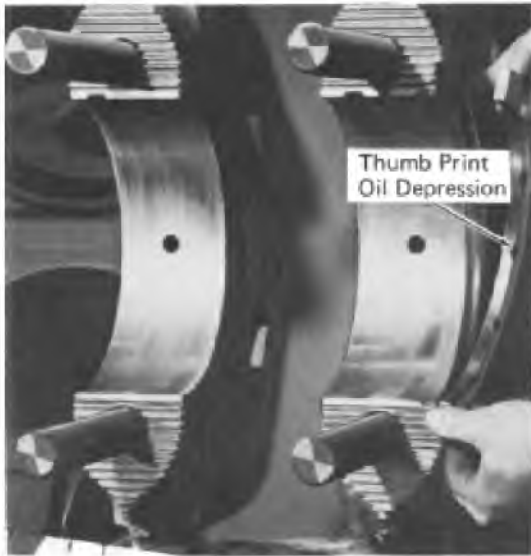
Fig. 6-3 - Applying Thrust Collar (16 & 20-Cyl.)
