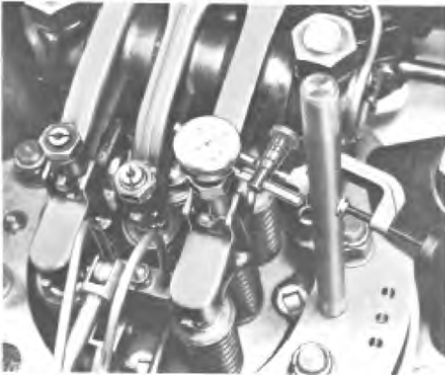
Fig. 15-7 -- Timing Exhaust Valves
