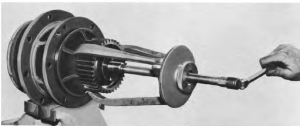
Fig. 10-10 - Drive Gear Removal
