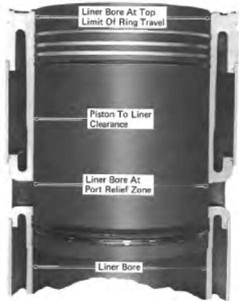
Fig. 4-6 - Liner Measurement Points
