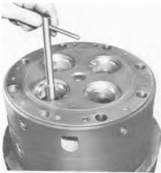
Fig. 2-11 - Tapered Pilot Installation
