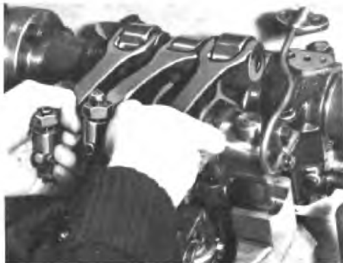
Fig. 5-24 - Rocker Arm Shaft Installation
