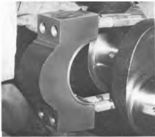
Fig. 6-4 - Main Bearing Shell And Cap
