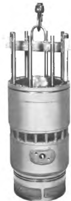
Fig. 5-18 - Liner Installation Using Liner Lifter
