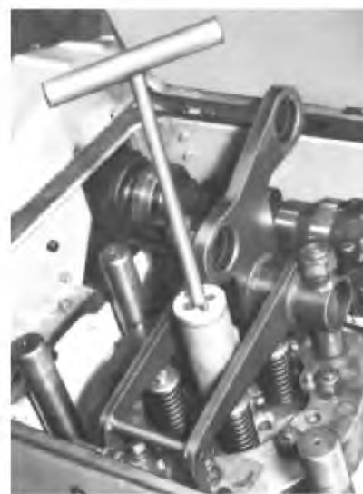
Fig. 5-11 - Piston Holding Tool Application
