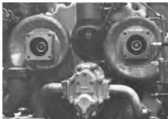
Fig. 10-6 - Water Pump Installation
