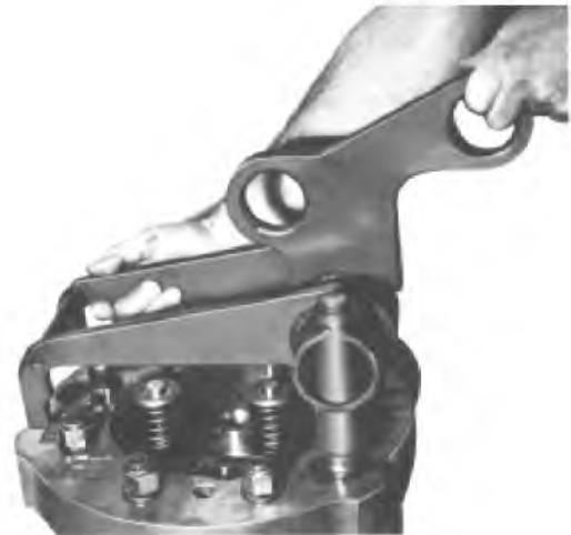
Fig. 5-29 - Lifting Clamp Application
