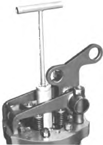
Fig. 5-30 - Piston Holding Tool Application
