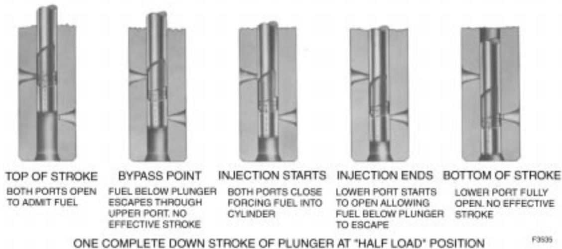
Figure 11-4. MUI Injector Fuel Flow
