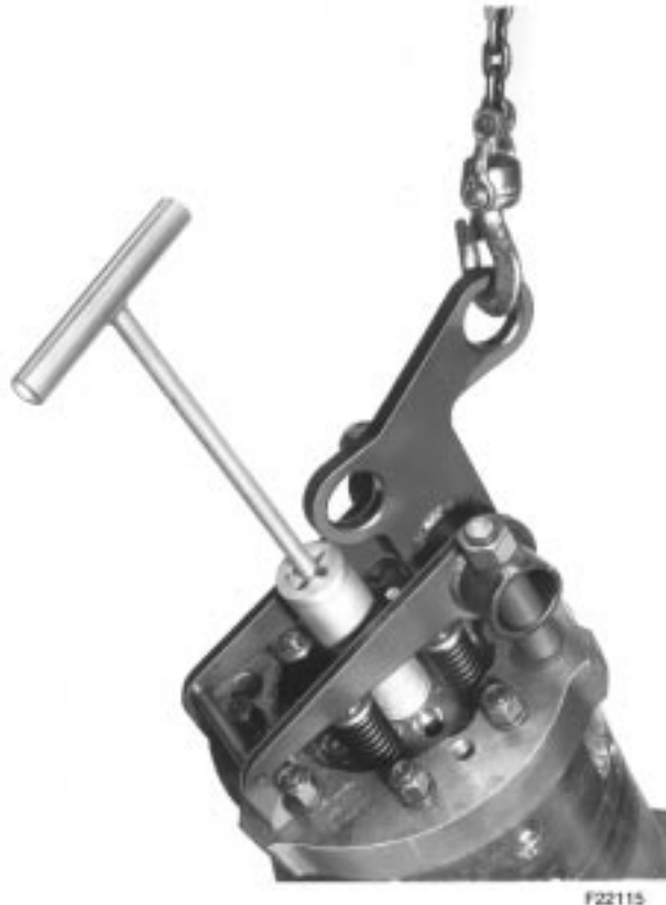
Figure 5-30. Power Assembly Installation With Clamp And Hoist
