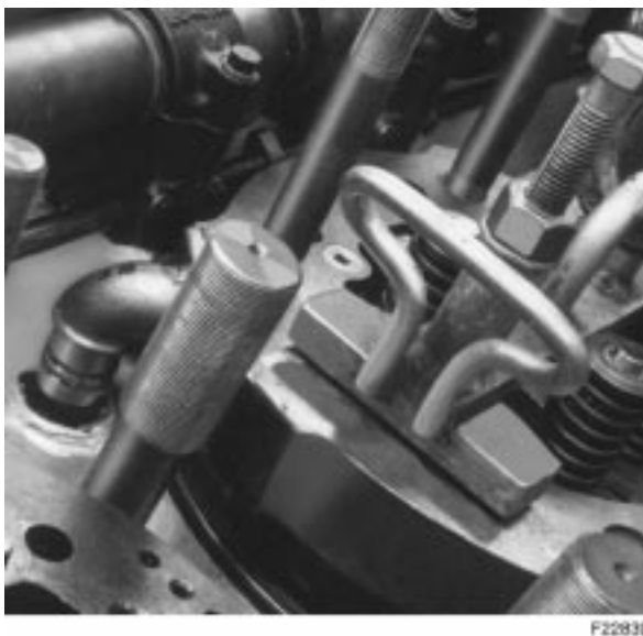
Figure 5-21. Water Discharge Elbow Alignment
