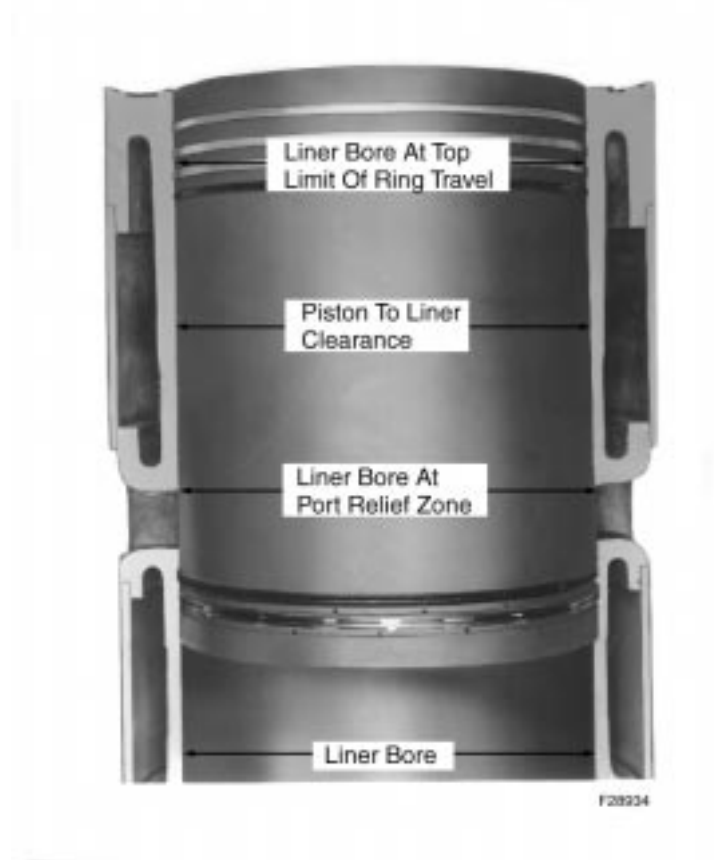
Figure 4-5. Liner Measurement Points
