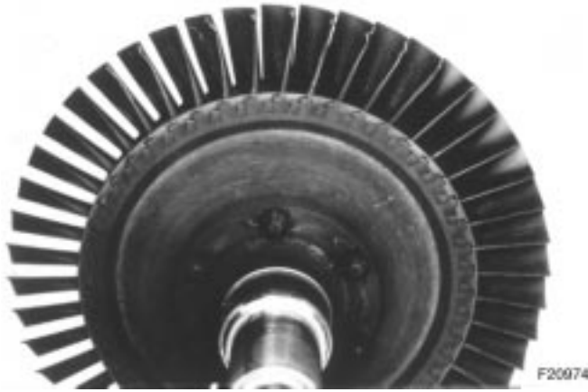
Figure 15-8 - Nicked Impeller Blades
