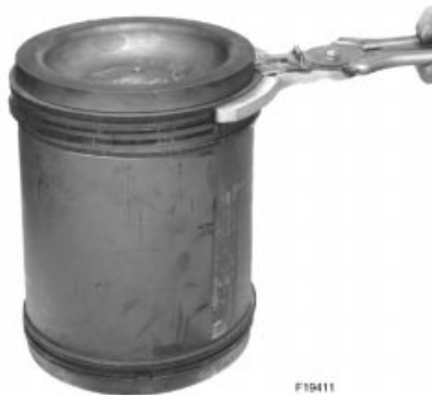
Figure 5-13. Installation Of Top Compression Ring
