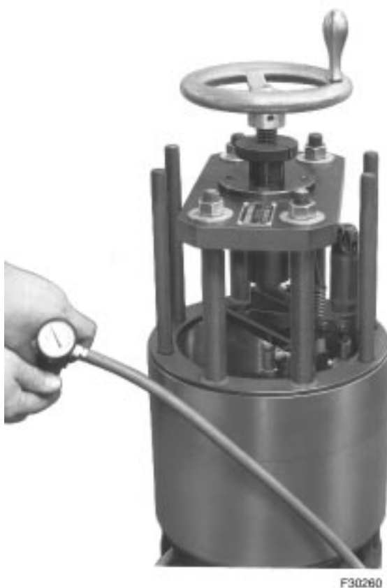
Figure 4-6. Application Of Liner Ridge Grinder
