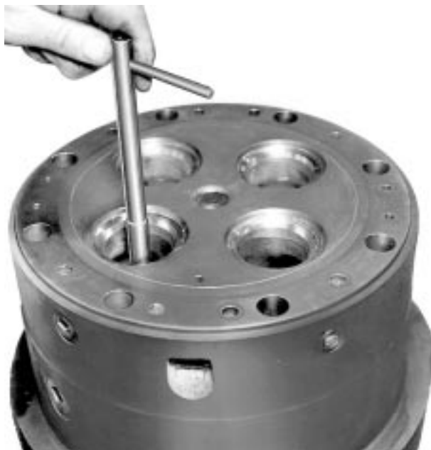
Figure 2-11. Tapered Pilot Installation
