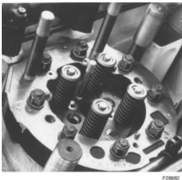
Figure 5-22. Head-To-Liner Nut Tightening Sequence
