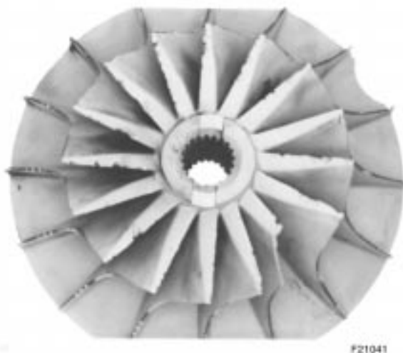
Figure 15-7 - Impeller Damaged By Foreign Material
