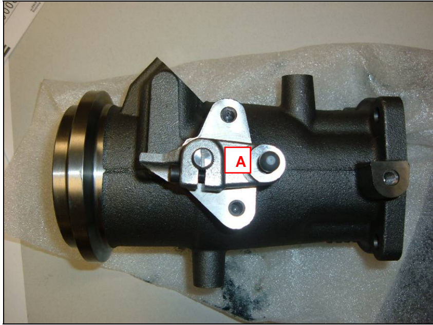
Figure 2 – Exhaust Flap Lever Adjustment
