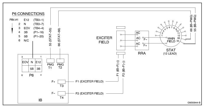
Figure 3-25 Interface Circuit Board Diagram
