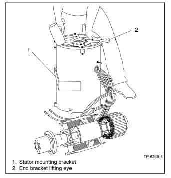
Figure 4-10 Attaching End Bracket on Stator
