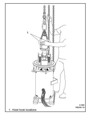
Figure 4-7 Rotor Removal
