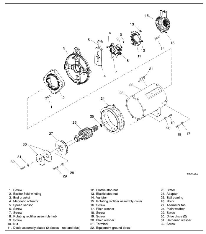
Figure 4-1 4PW and 4QW Alternator Components, 20-60 kW
