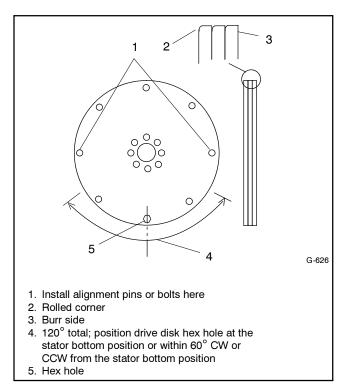
Figure 4-15 Aligning and Mounting Drive Disks
