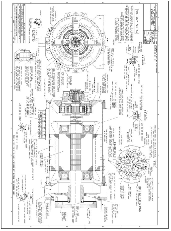
Figure 4-25 4UAW Alternator Components, 180-300 kW
