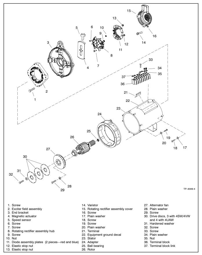
Figure 4-2 4SW, 4VW, and 4UAW Alternator Components, 60 kW IMS-300 kW
