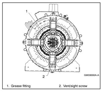
Figure 4-16 Applying Grease to UA Alternator
