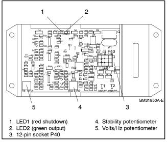
Figure 3-5 Voltage Regulator Features
