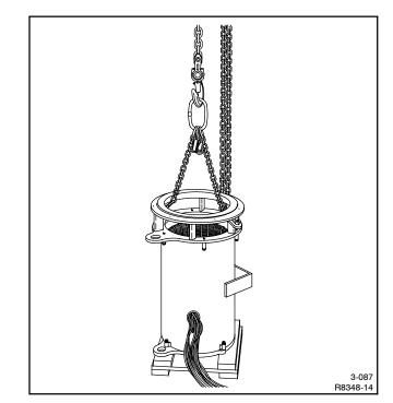
Figure 4-12 Supporting Alternator Assembly
