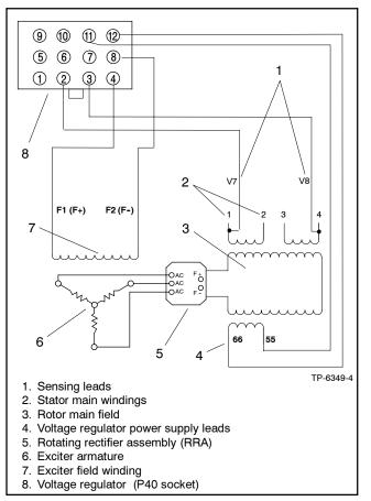
Figure 3-7 Voltage Regulator Connection
