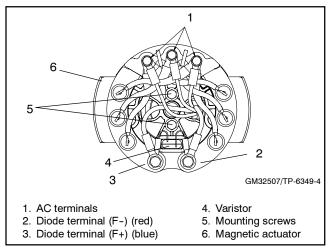
Figure 4-3 Rotating Rectifier Assembly Hub and Components
