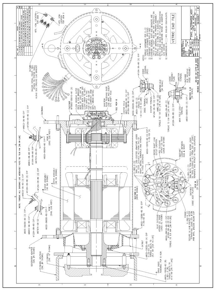
Figure 4-23 4PW and 4QW Alternator Components, 20-60 kW
