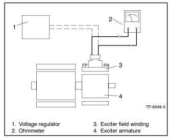
Figure 3-8 Exciter Field Winding Resistance Test
