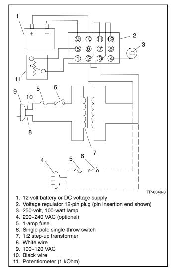
Figure 3-3 Voltage Regulator Test with User-Fabricated Adapter Harness
