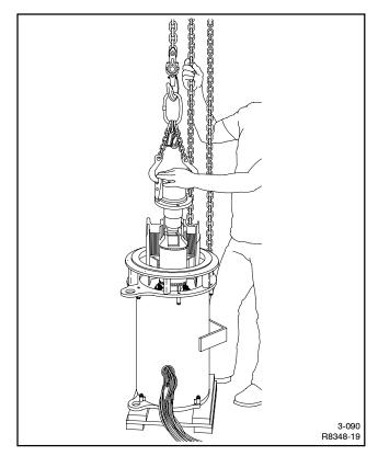
Figure 4-14 Installing Rotor
