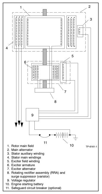
Figure 1-1 WF Alternator
