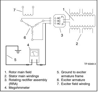
Figure 3-11 Megohmmeter Connections on Exciter Armature
