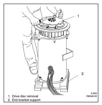
Figure 4-6 Alternator Support, Drive Discs, and Fan Removal
