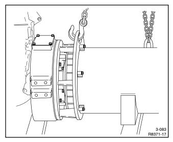
Figure 4-19 Aligning Adapter to Flywheel Housing
