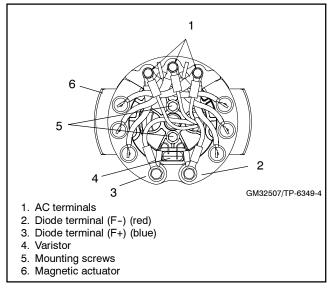
Figure 4-20 Rotating Rectifier Assembly Hub and Components
