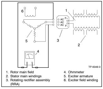
Figure 3-10 Exciter Armature Resistance Test
