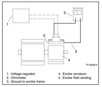
Figure 3-9 Megohmmeter Connections on Exciter Field Winding
