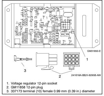
Figure 3-4 Voltage Regulator Adapter Harness
