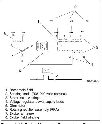
Figure 3-19 Stator Ohmmeter Connections, Single Phase
