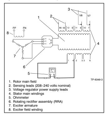
Figure 3-17 Stator Ohmmeter Connections, 3-Phase
