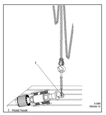
Figure 4-13 Hoisting Rotor
