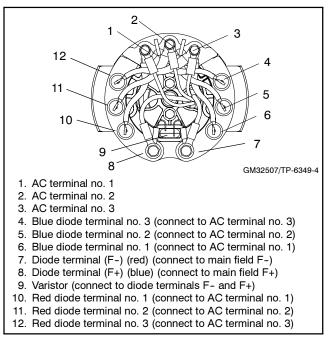
Figure 4-21 Rotating Rectifier Assembly Hub Electrical Connections
