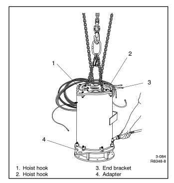
Figure 4-9 Removing Alternator Adapter
