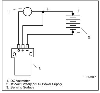
Figure 3-22 Speed Sensor Test
