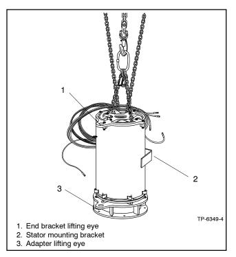
Figure 4-11 Aligning Adapter and Stator
