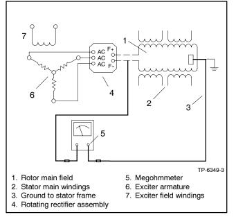
Figure 3-15 Megohmmeter Connections on Rotor Main Field
