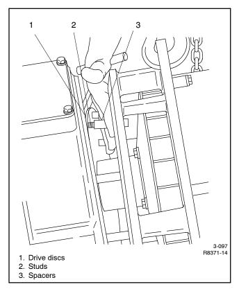
Figure 4-18 Installing Spacers
