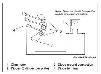
Figure 3-13 Diode Assembly Plate (part of RRA) Test
