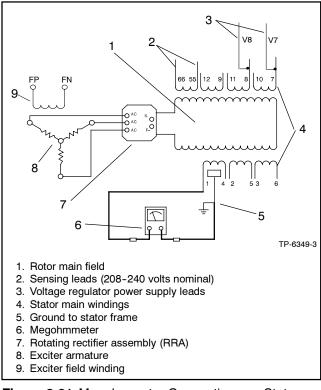
Figure 3-21 Megohmmeter Connections on Stator, Three Phase
