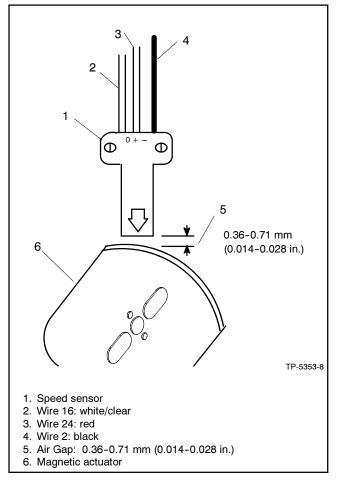
Figure 4-22 Speed Sensor Air Gap
