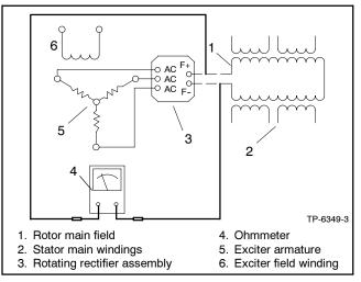
Figure 3-14 Rotor Resistance Test
