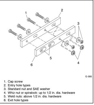
Figure 2 Acceptable Hardware Combinations
