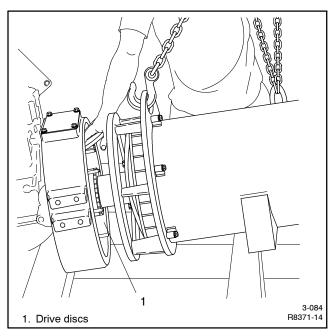
Figure 4-5 Separating Generator and Engine
