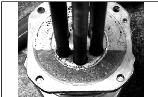
Figure 7 Heater Showing Coolant Line from Horizontal Mounting
