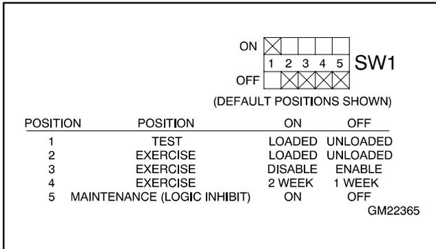
**Figure 3** DIP Switches
