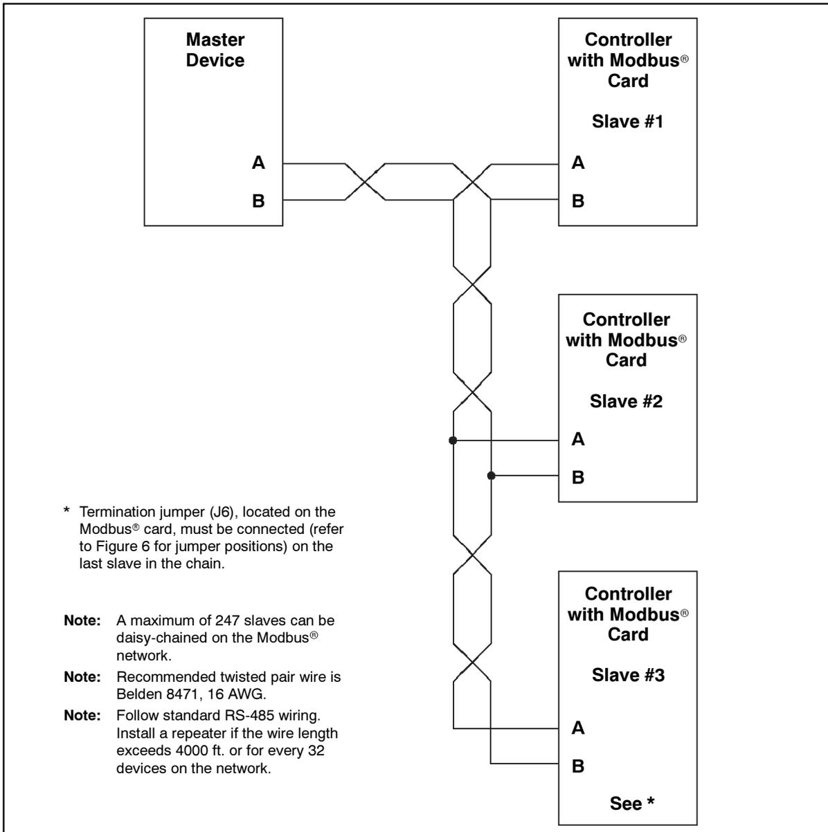
**Figure 2** RS-485 Multi-Drop Connection
