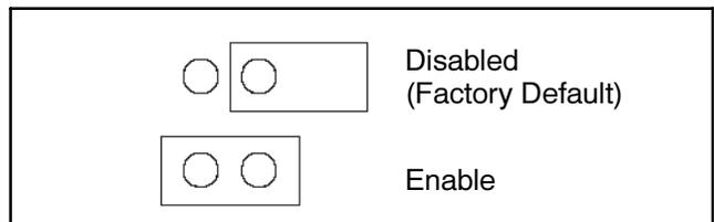
**Figure 6** Jumper J6 (enable only on the last device in the network)
