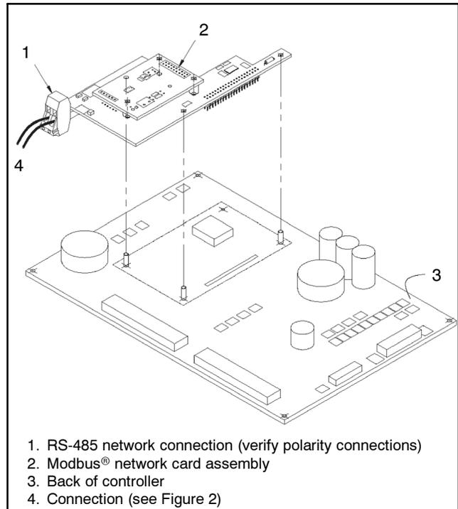
**Figure 1** Location of Modbus® Card on Controller
