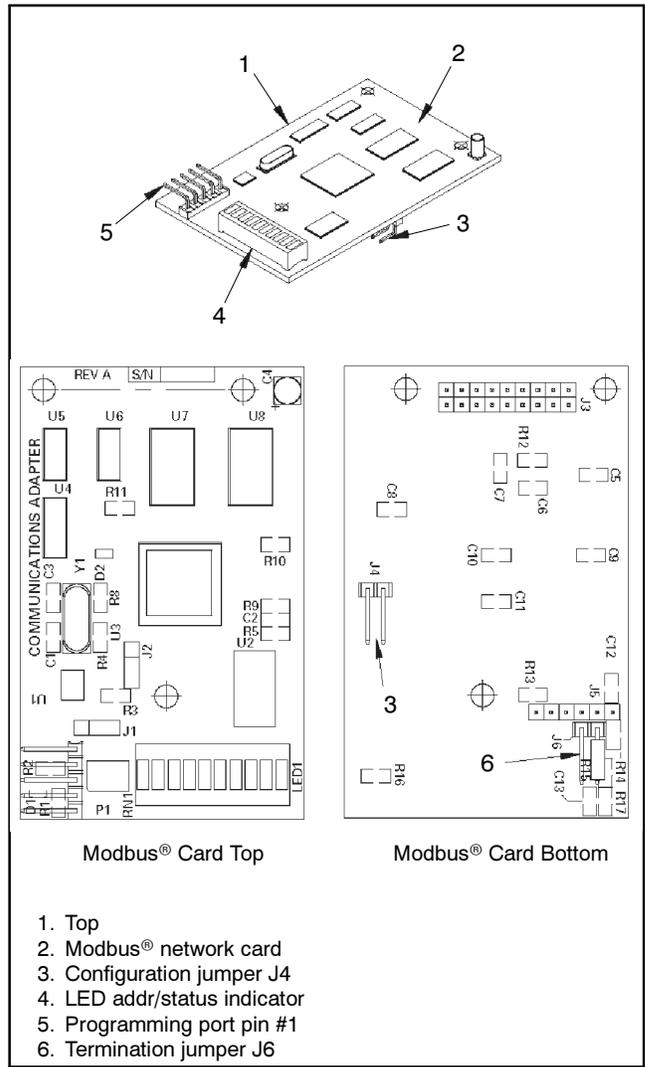
**Figure 5** Modbus® Network Card
