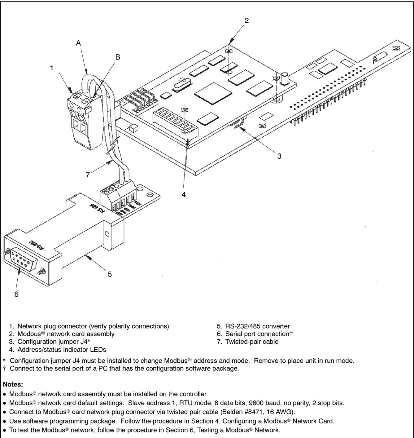
**Figure 9** Connections to Configure and Test Modbus® Card
