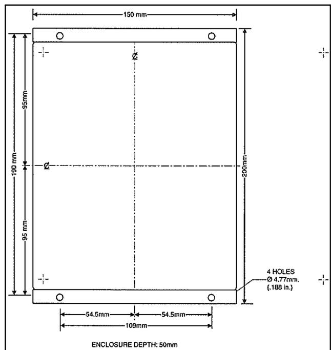
Figure 7 Mounting Dimensions
