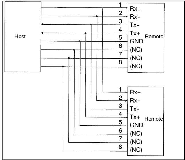
**Figure 46** Connections, CIM (Host) to TSC 800 Controllers (Remotes)
