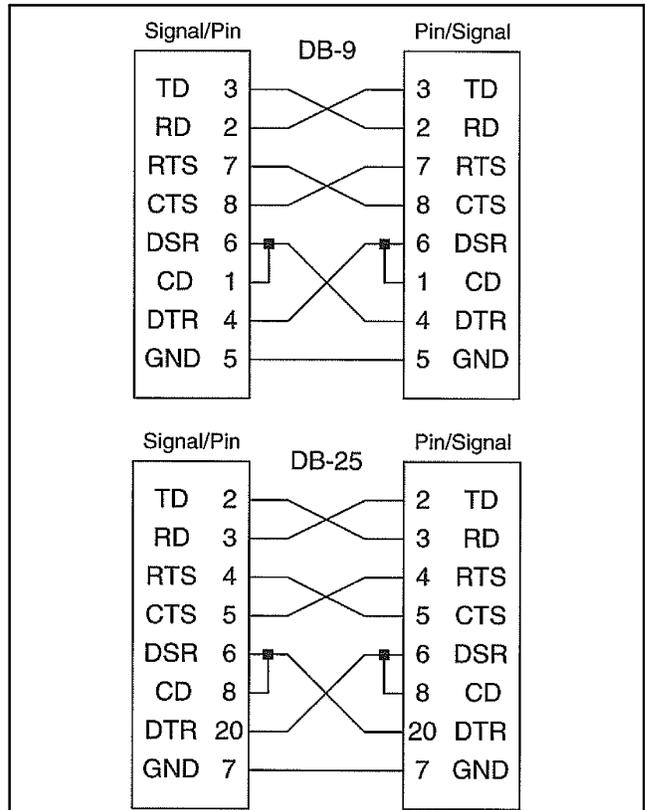
**Figure 44** Null Connection, Model-Converter
