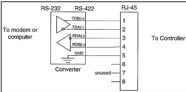
**Figure 43** Wiring, RS-422 to RJ-45
