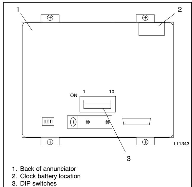
**Figure 20** Annunciator DIP Switches
