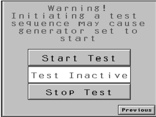
**Figure 19** Test Warning Screen
