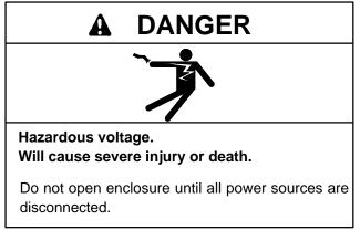
Hazardous voltage can cause severe injury or death. De-energize both normal and emergency power sources before proceeding. Move generator master switch on controller to OFF position and disconnect battery negative (–) before working on transfer switch! Turn the transfer switch selector switch to the OFF position.
