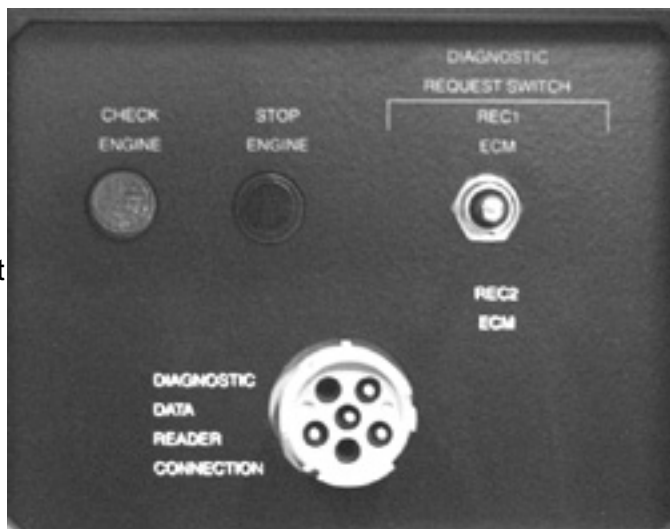
Diagnostic panel for series 2000 and 4000 models
