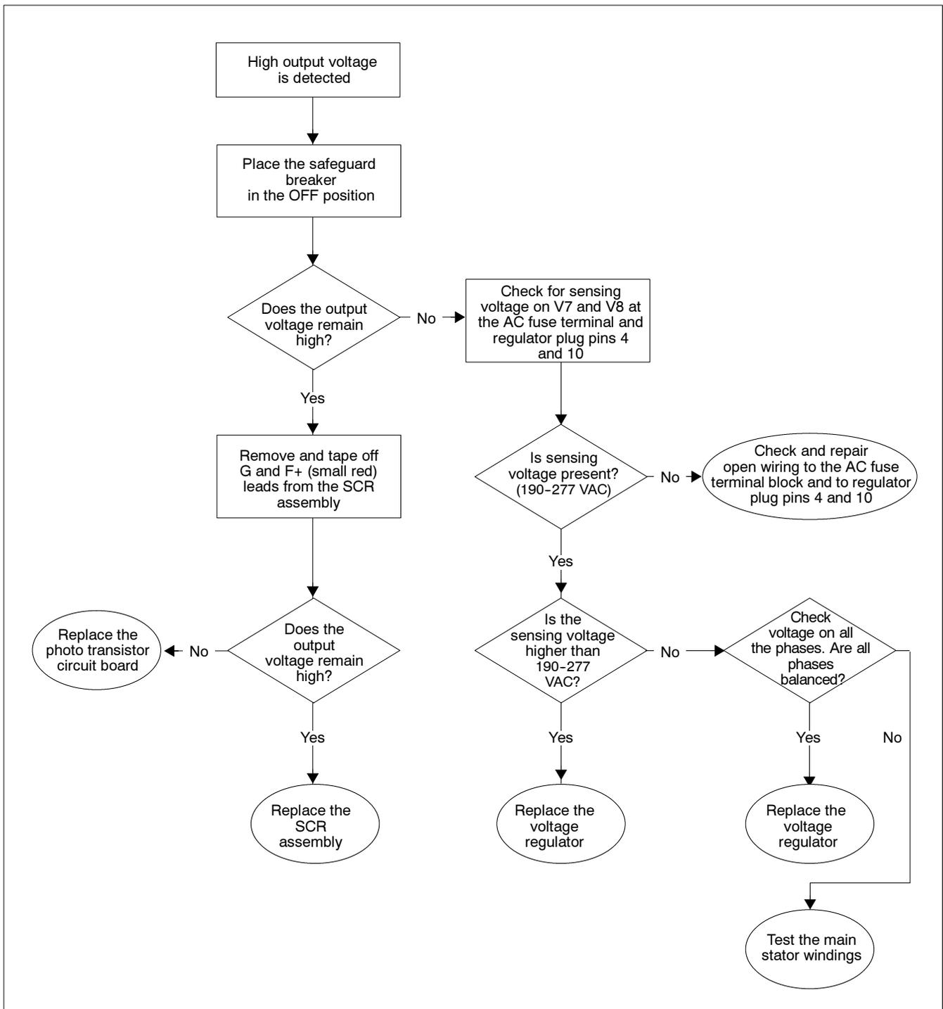
**Figure 2** Troubleshooting Flowchart for High Output Voltage
