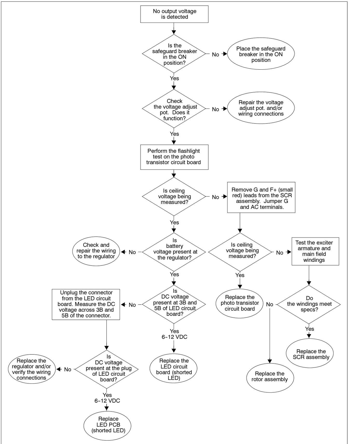
**Figure 1** Troubleshooting Flowchart for No Output Voltage
