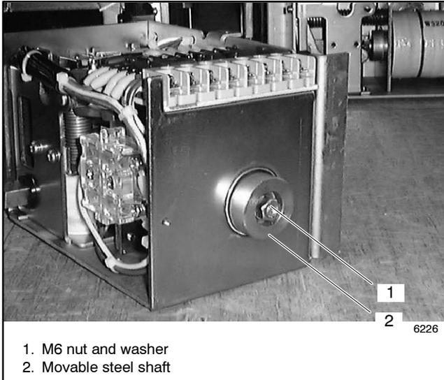
**Figure 6-14** Movable Steel Shaft, 100-400 Amp Models
