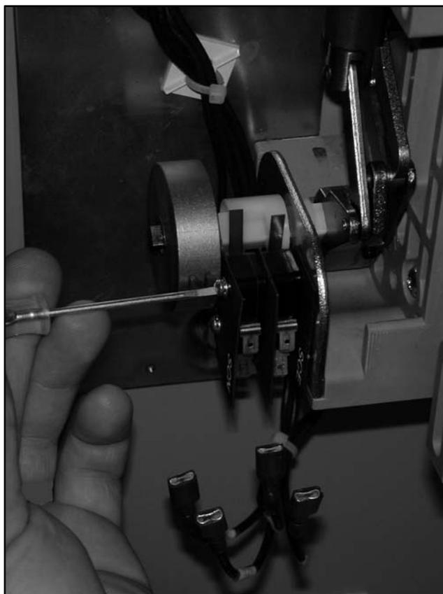
**Figure 5-13** Microswitch Installation
