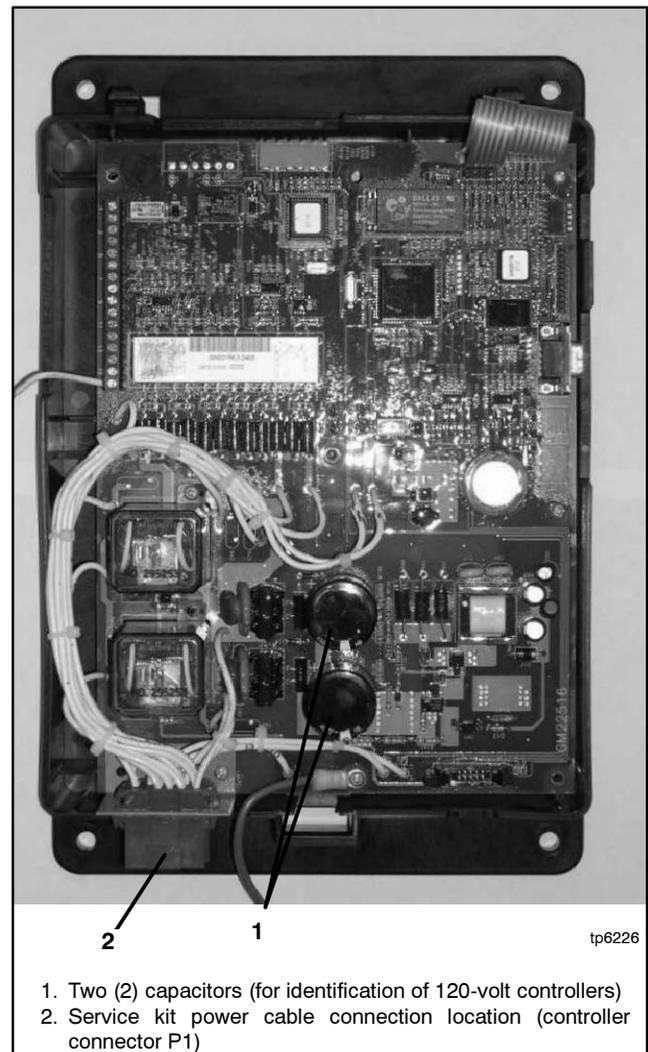
**Figure 3-6** 120-Volt Circuit Board with 120 VAC Power Connection Location (P1)
