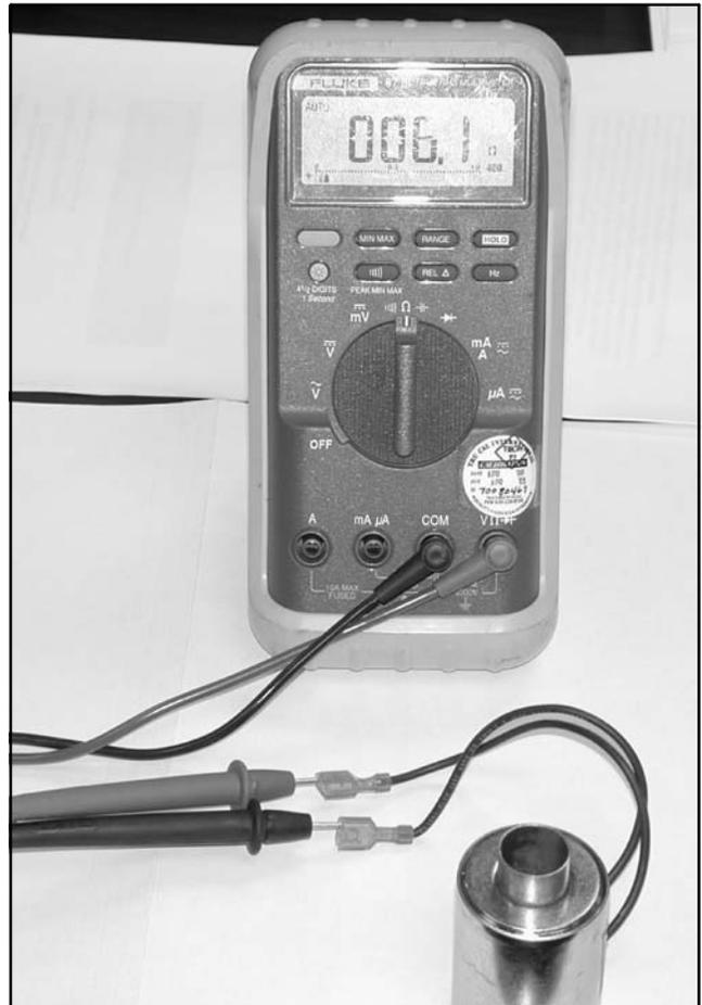
**Figure 5-15** Checking Coil Resistance
