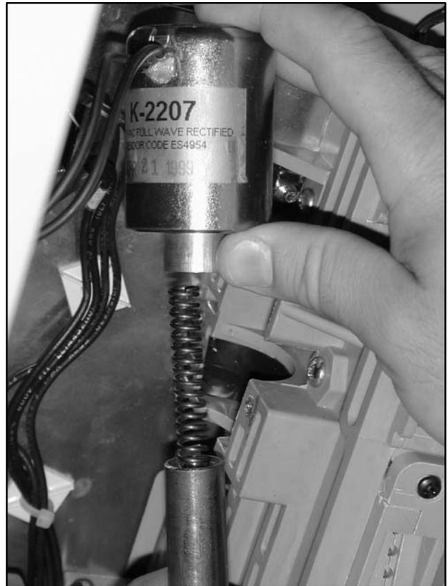
**Figure 5-18** Spring and Plunger Assembly
