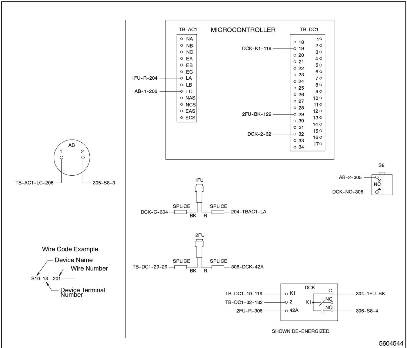
Figure 5-72. Wiring Diagram—Option KD-31-DA
