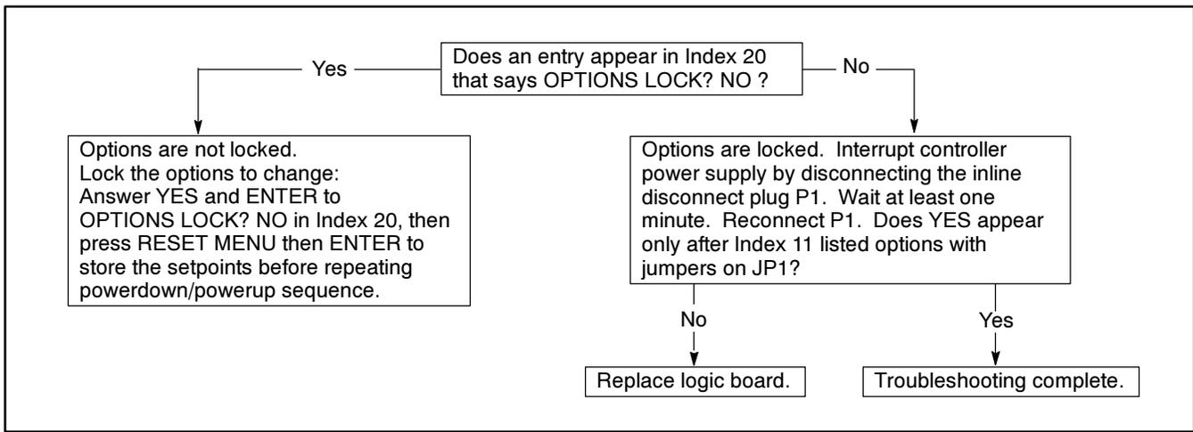
**Figure 4-17. Troubleshooting—YES appears in Index 11 when a jumper for that option is not installed**
