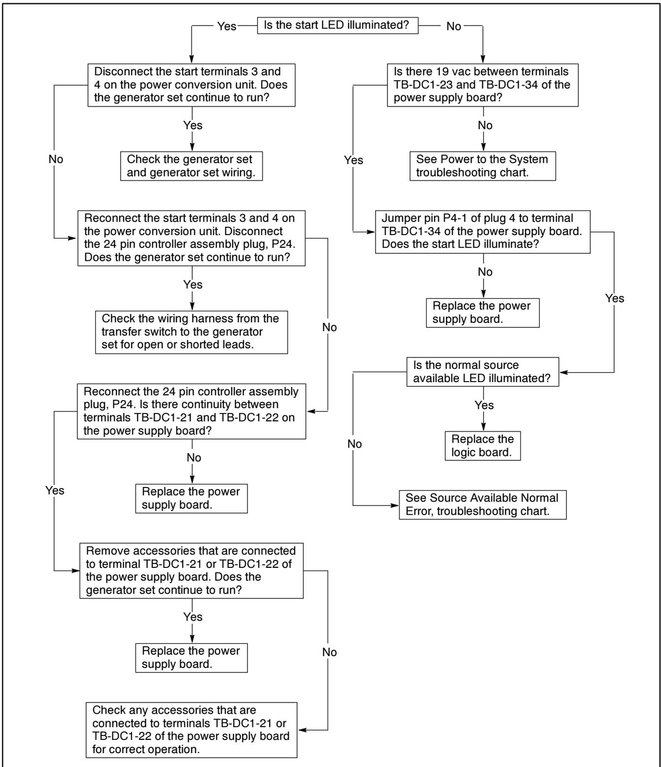
**Figure 4-11. Troubleshooting—Engine operates when it should not**
