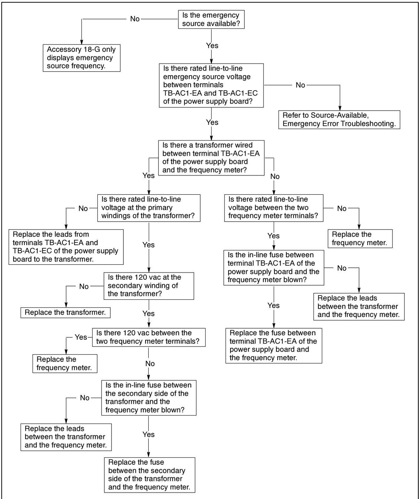
**Figure 5-37. Troubleshooting—Option KD-18-G, Meter will not display frequency**
