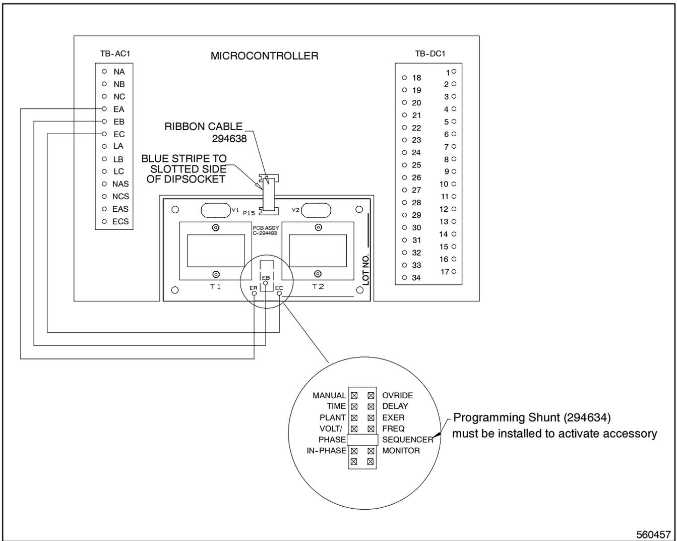
**Figure 5-3. Wiring Diagram—Three-phase emergency source sensing, Option KD-05-K**
