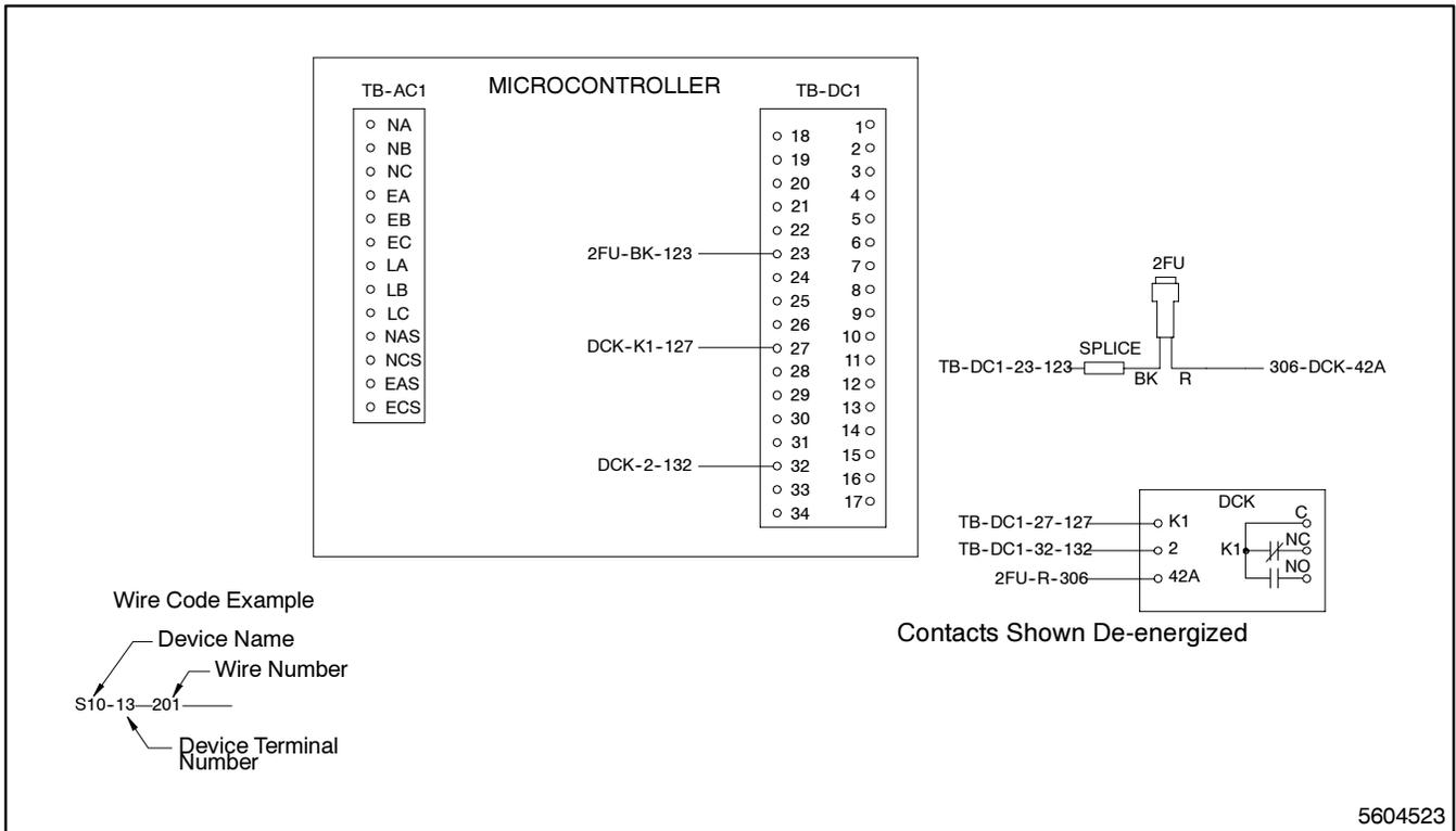
**Figure 5-19. Wiring Diagram—Option KD-14-J**
