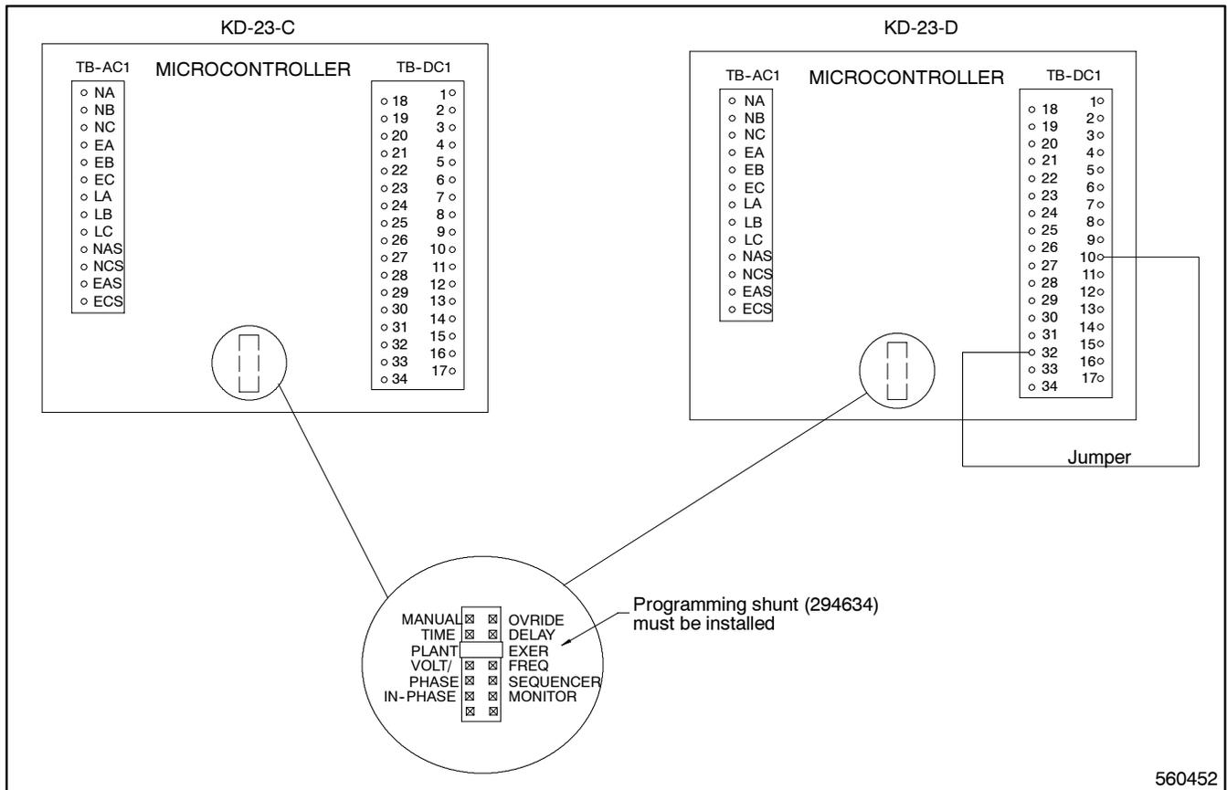
Figure 4-25. Wiring Diagram—Plant exerciser, option KD-23-C and KD-23-D
