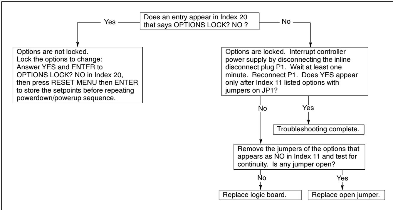
**Figure 4-18. Troubleshooting—NO appears in Index 11 when a jumper for that option is installed**
