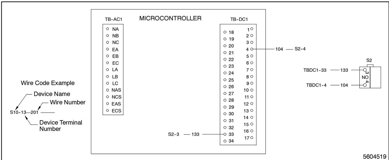
Figure 5-12. Wiring Diagram—Time delay override, Option KD-08-C
