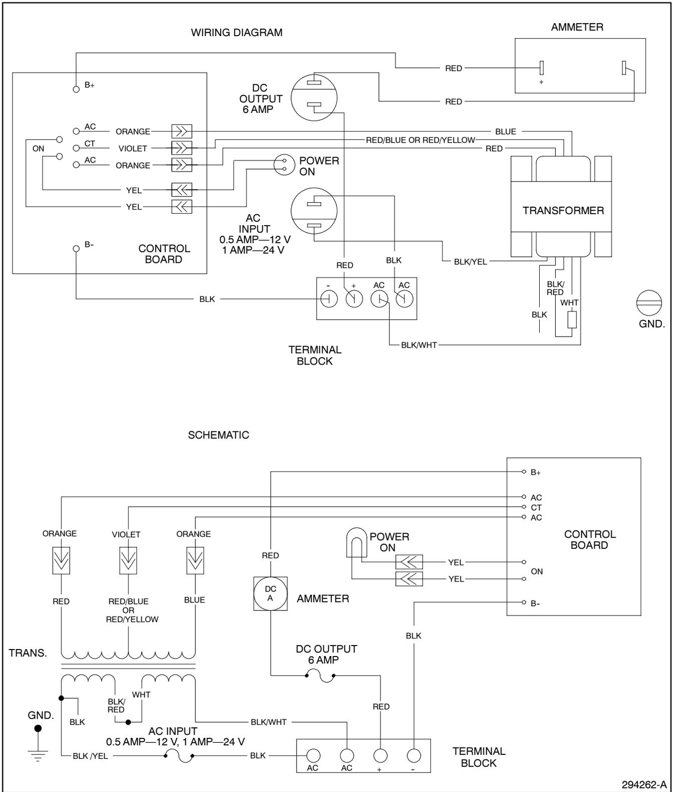
Figure 5-60. Wiring Diagram—Option KD-24, Battery charger 240-volt input
