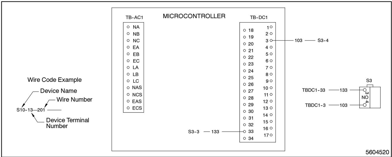
**Figure 5-13. Wiring Diagram—Time delay override, Option KD-08-D**
