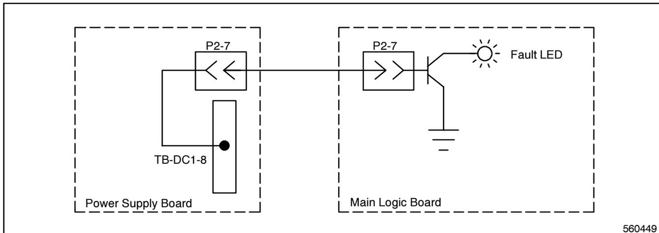
Figure 4-9. Wiring Diagram—Fault #1 or Fault #2 message
