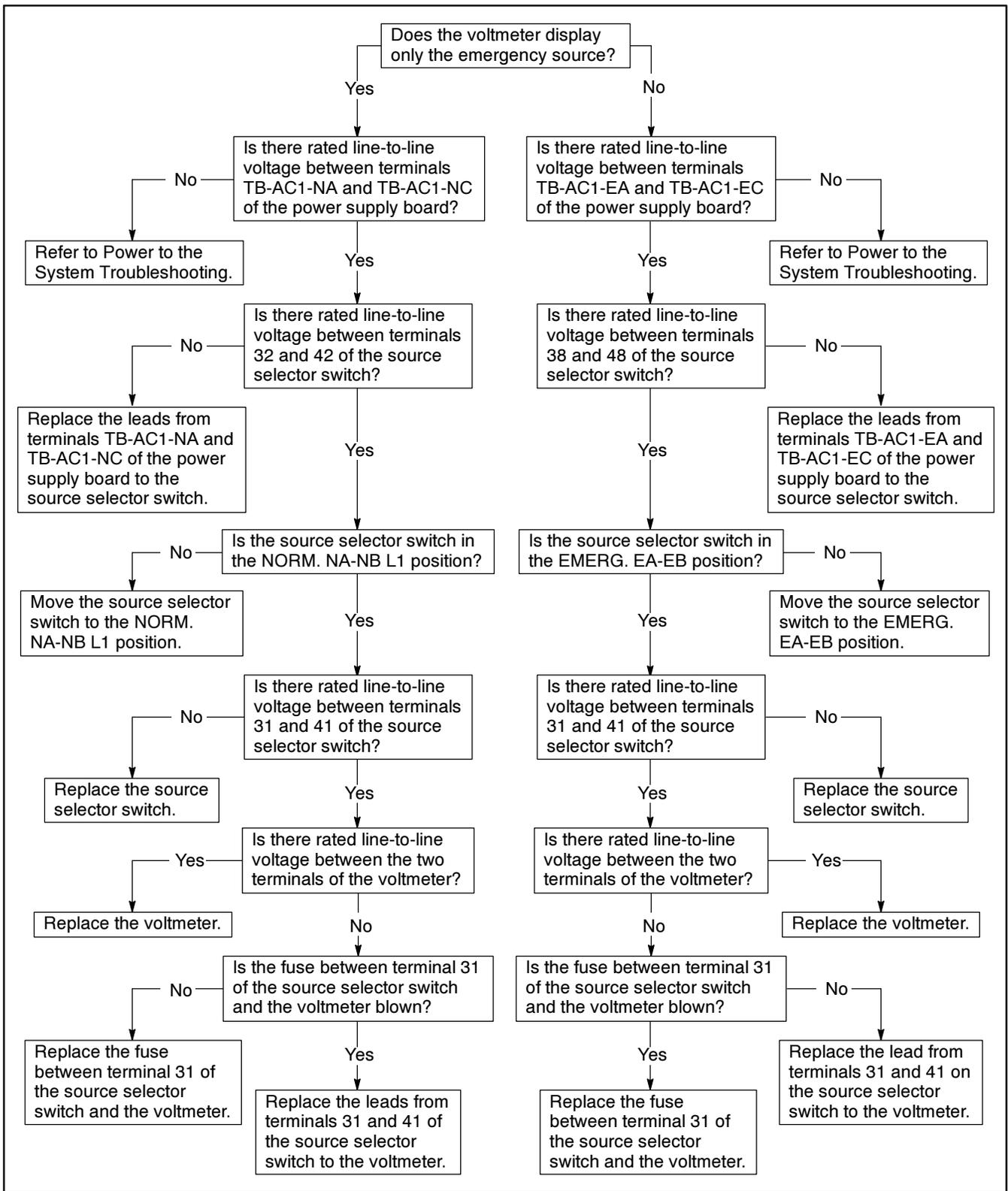
**Figure 5-42. Troubleshooting—Option KD-18-J, Voltmeter is not functioning**
