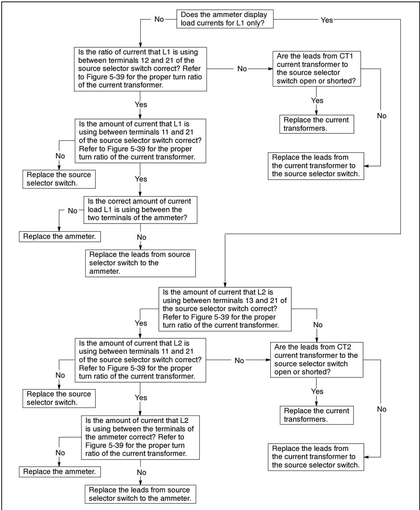
**Figure 5-43. Troubleshooting—Option KD-18-J, Ammeter is not functioning**
