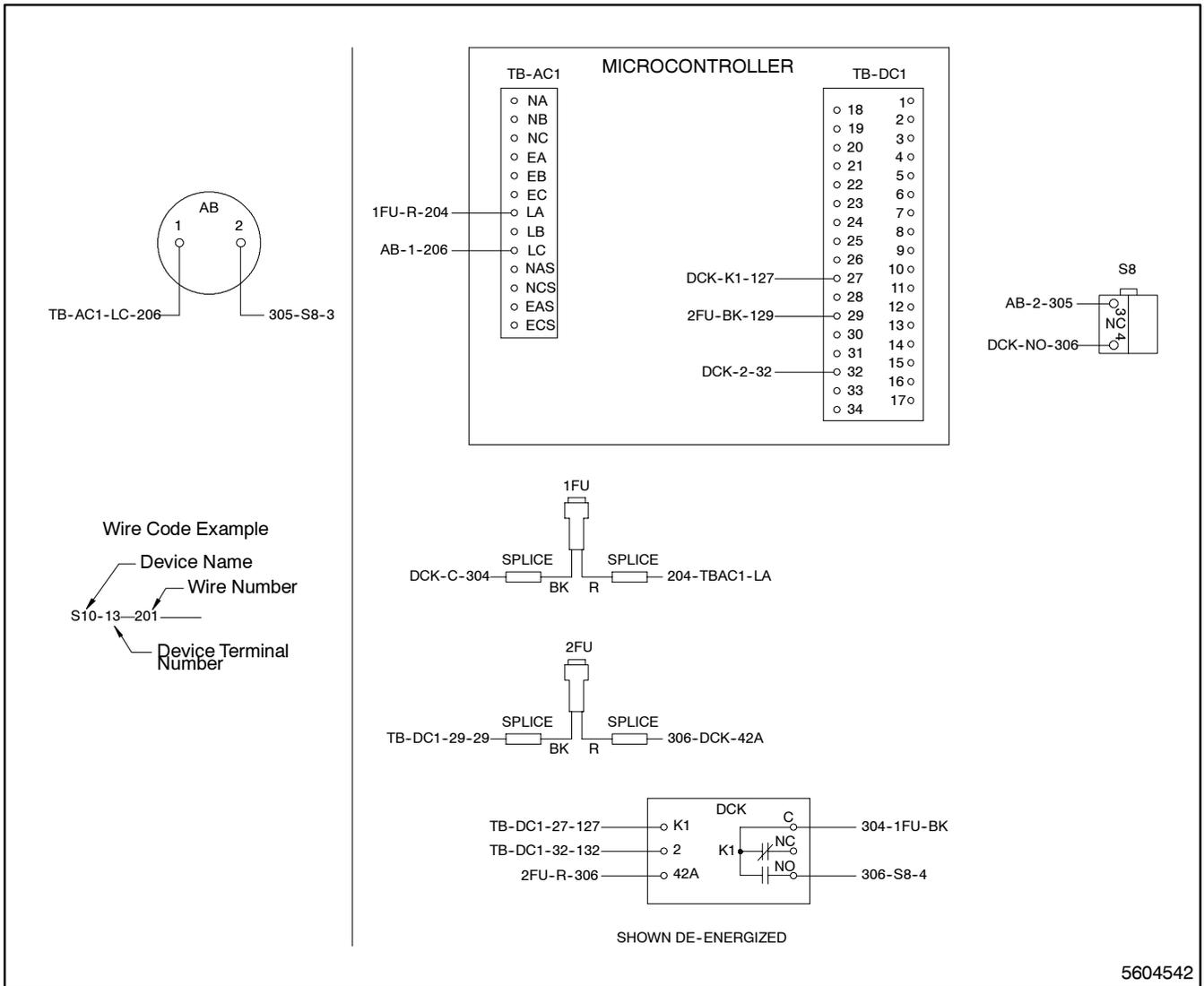
**Figure 5-70. Wiring Diagram—Option KD-31-BA**
