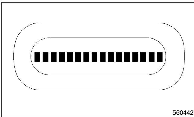
**Figure 4-2. MATS LCD display during a lamp test**
