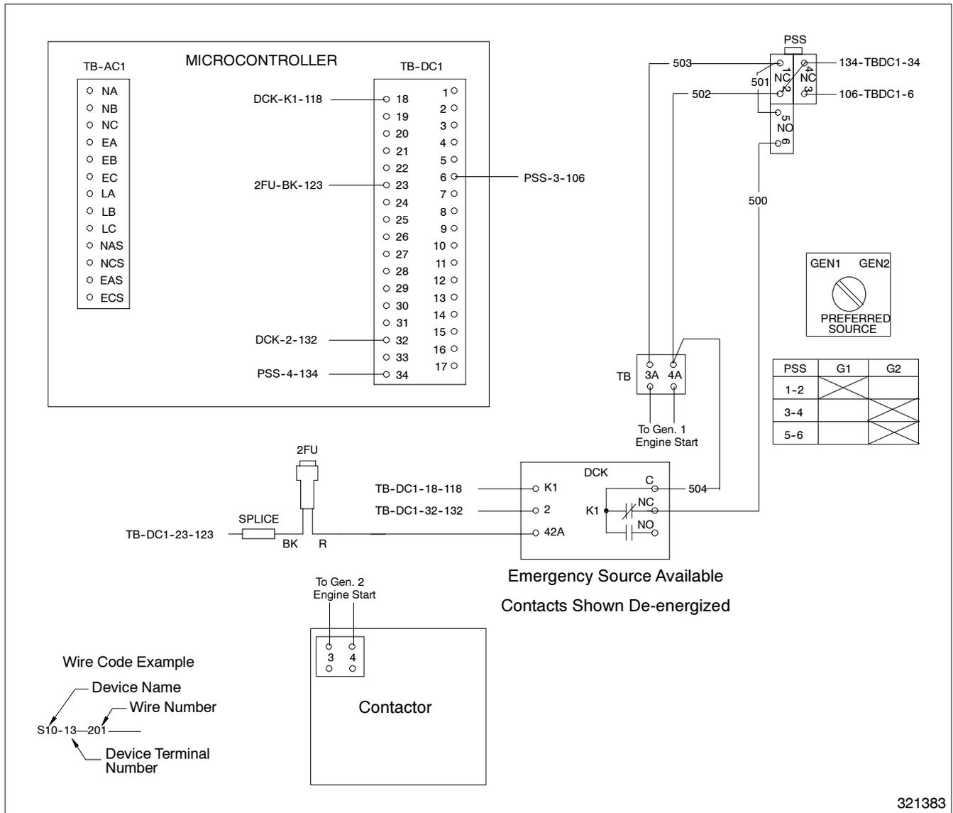
Figure 5-16. Wiring Diagram—Preferred source switch, Option KD-10
