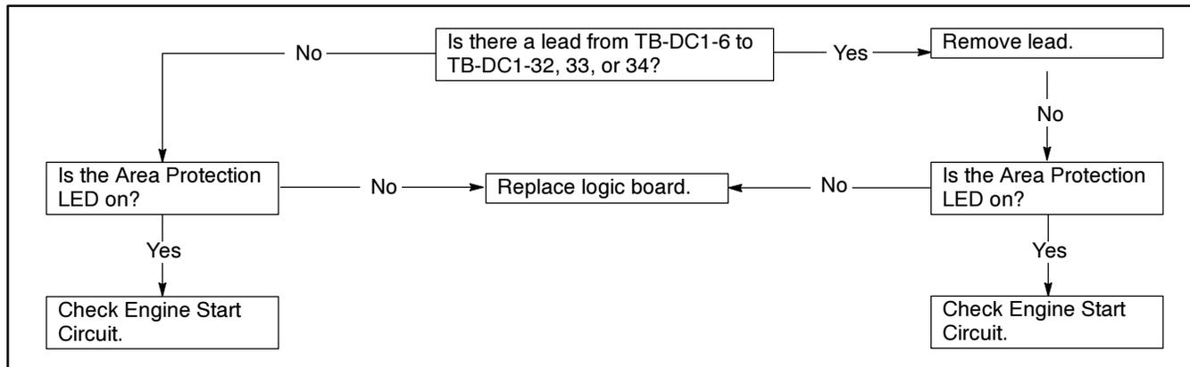
Figure 4-13. Troubleshooting—Area protection does not turn on
