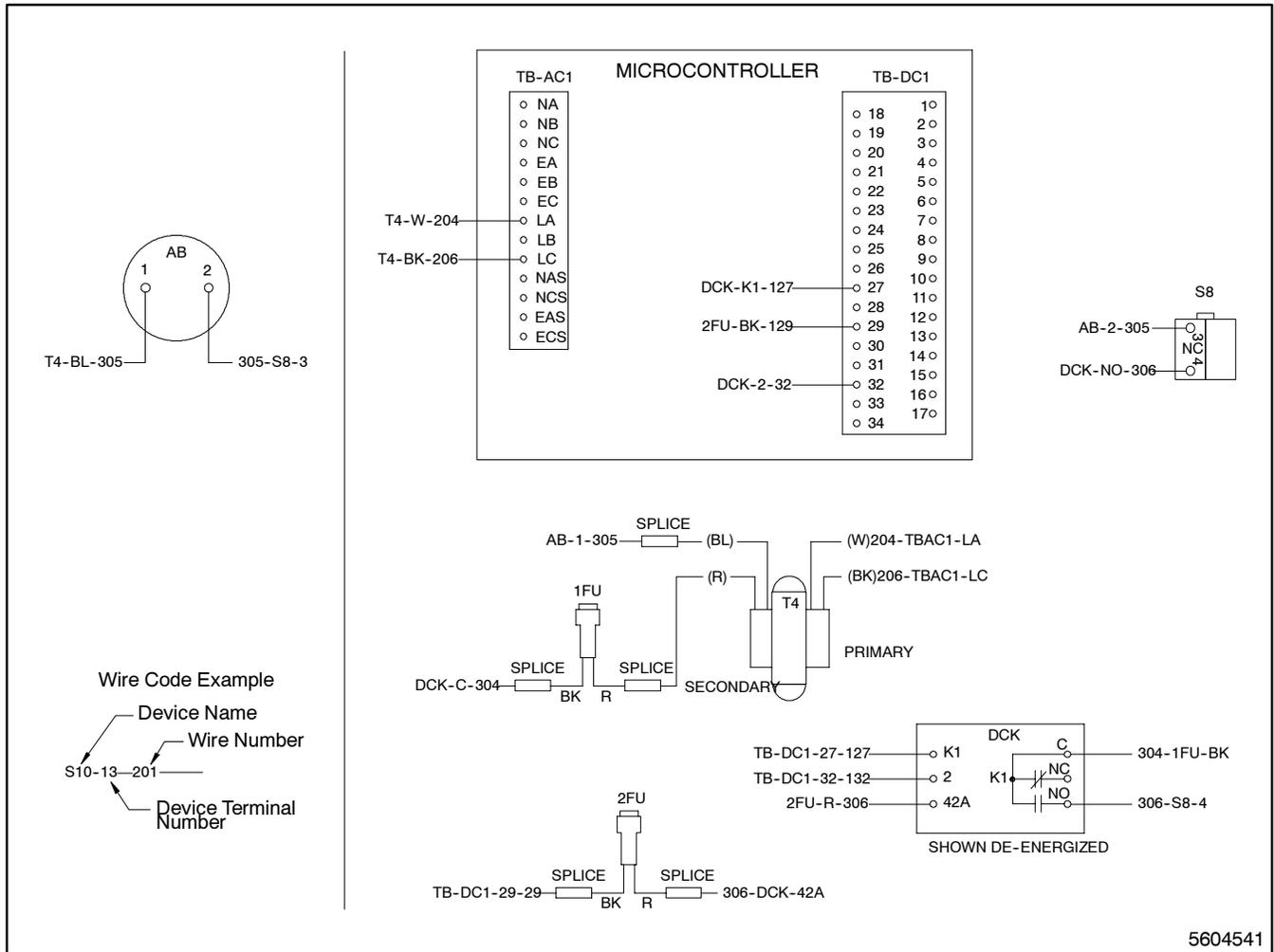
Figure 5-69. Wiring Diagram—Option KD-31-B
