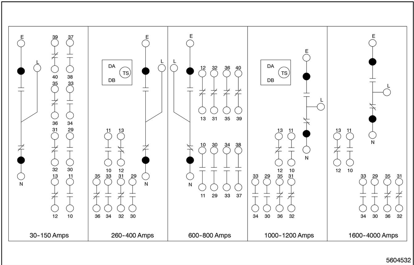
**Figure 5-30. Main shaft auxiliary contacts location**
