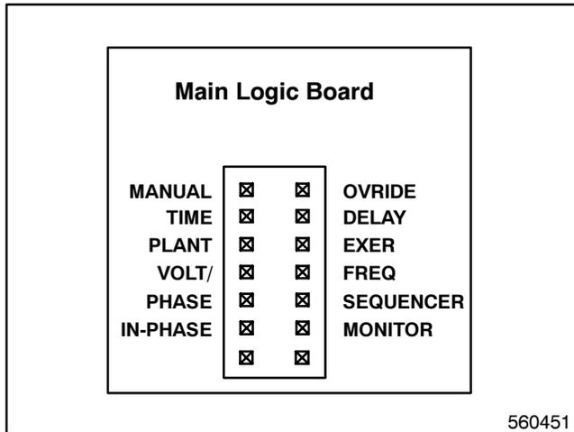
**Figure 1-5. MATS Logic Board Accessory Programming Shunts**
