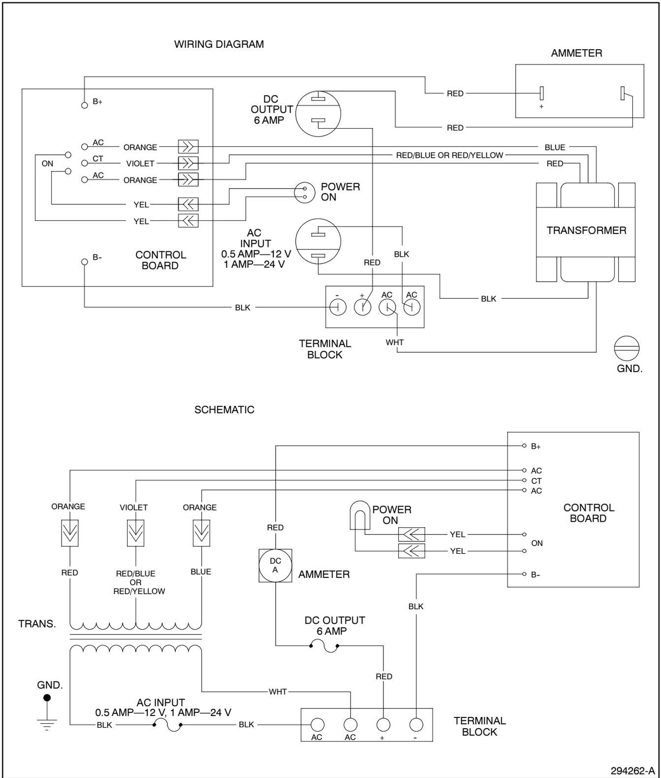
**Figure 5-59. Wiring Diagram—Option KD-24, Battery charger 220-volt input**
