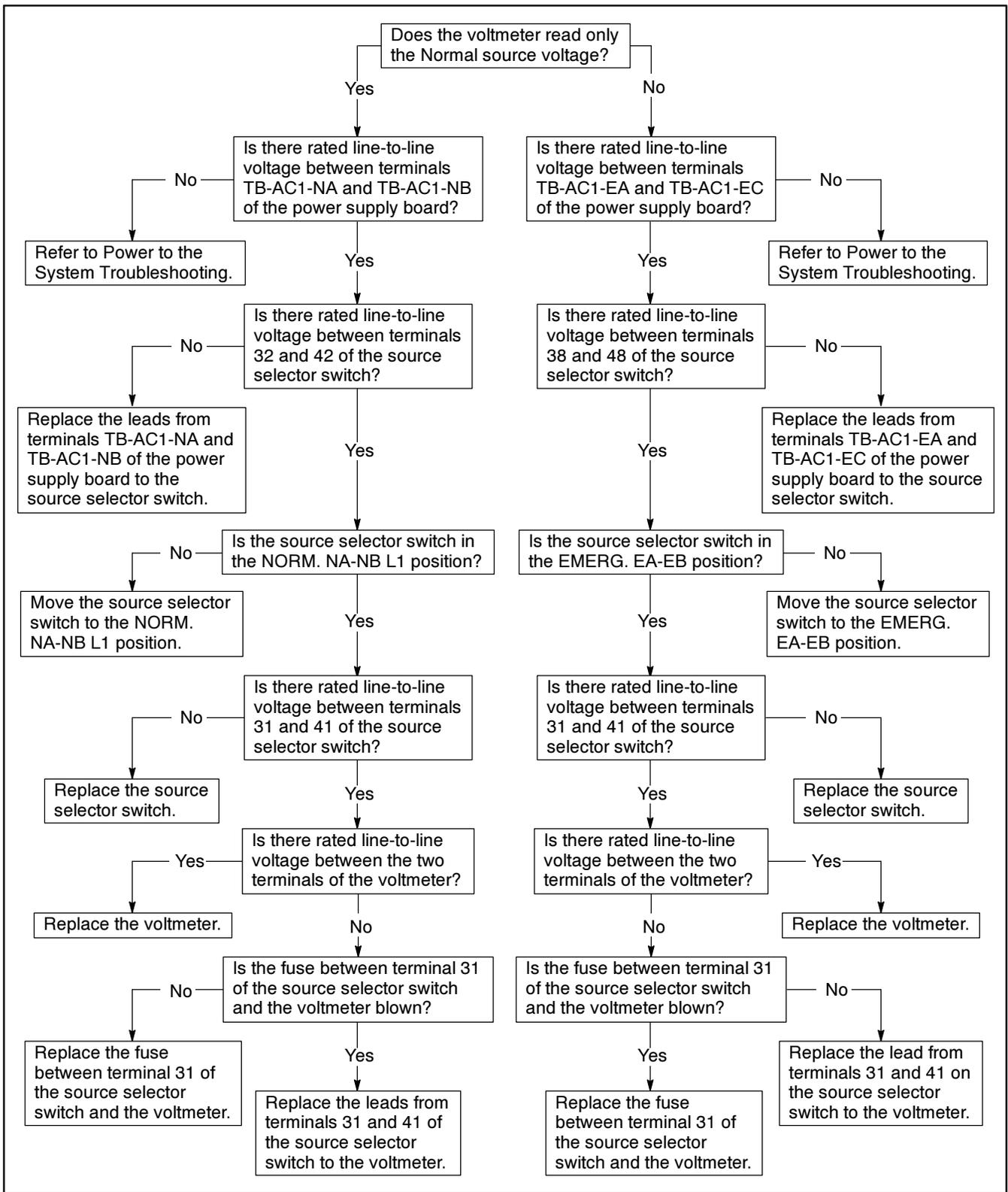
**Figure 5-40. Troubleshooting—Option KD-18-J, Voltmeter is not functioning**
