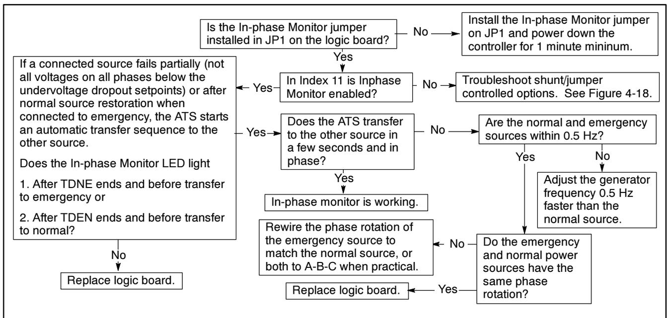
Figure 4-20. Troubleshooting—Inphase monitor, does not work
