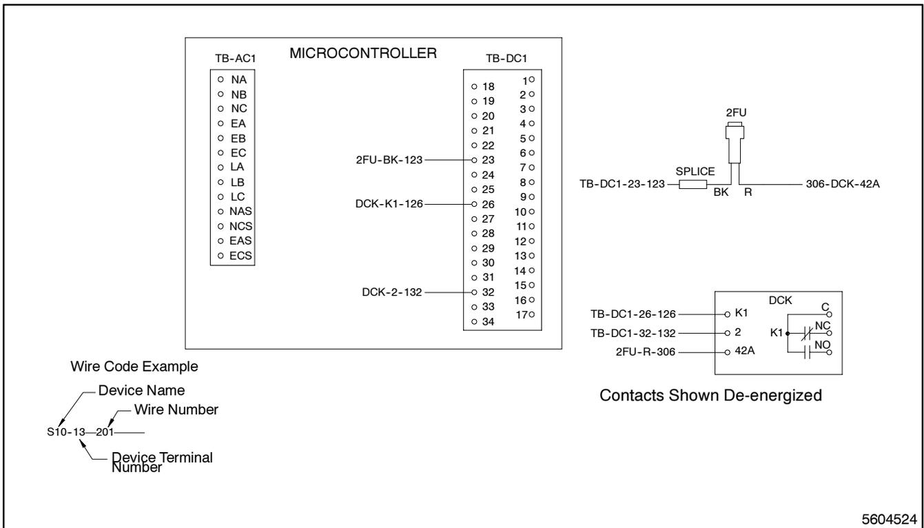
**Figure 5-20. Wiring Diagram—Option KD-14-K**
