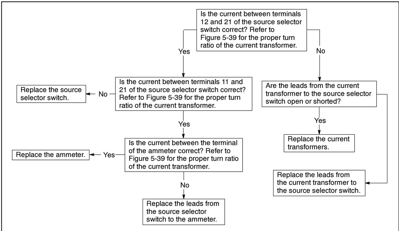
Figure 5-41. Troubleshooting—Option KD-18-J, Ammeter is not functioning
