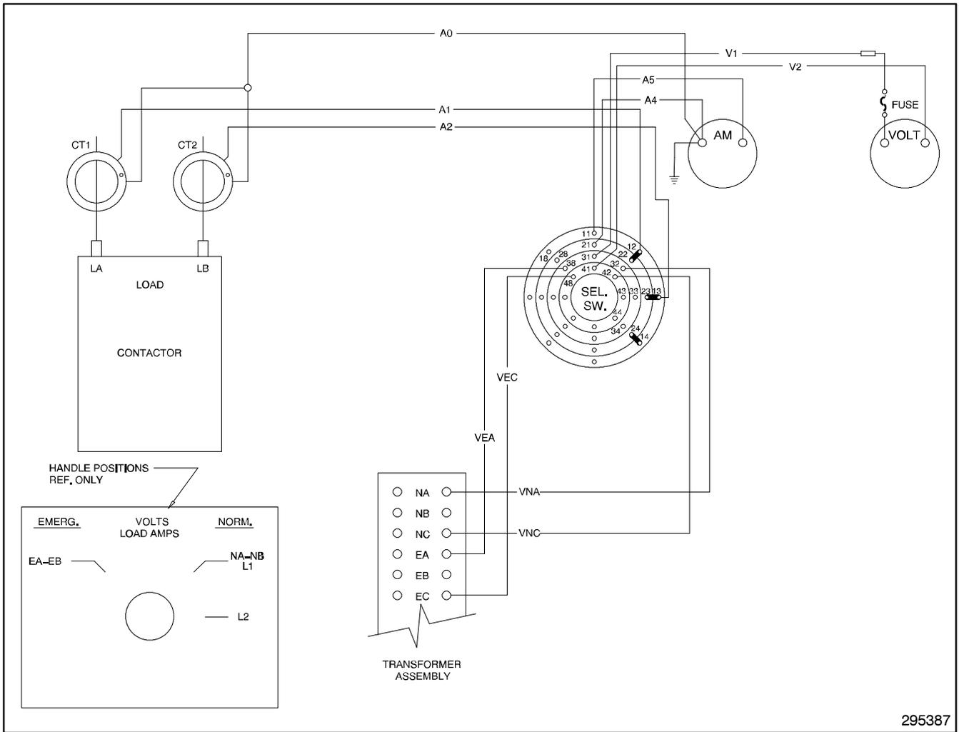
Figure 5-34. Wiring Diagram—Option KD-18-J, Analog volt and amp meter
