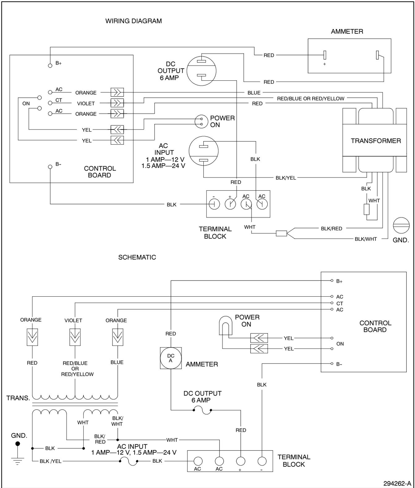
**Figure 5-58. Wiring Diagram—Option KD-24, Battery charger 120-volt input**
