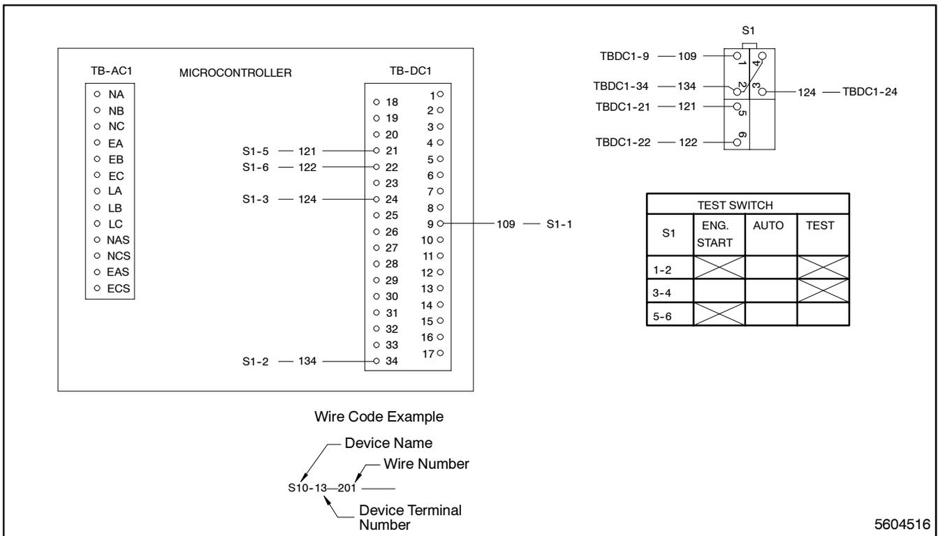
**Figure 5-4. Wiring Diagram—Test Switches, Options DD-06-N, -P, -R, -T**
