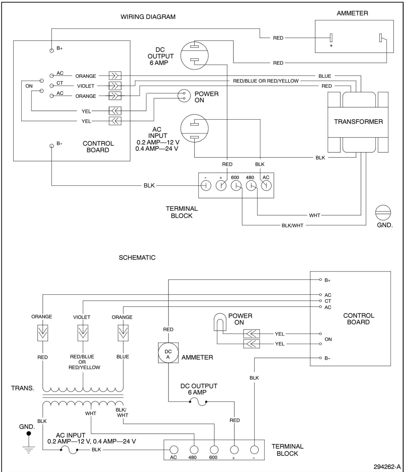
Figure 5-58. Wiring Diagram—Option DD-24, Battery Charger 480/600-Volt Input
