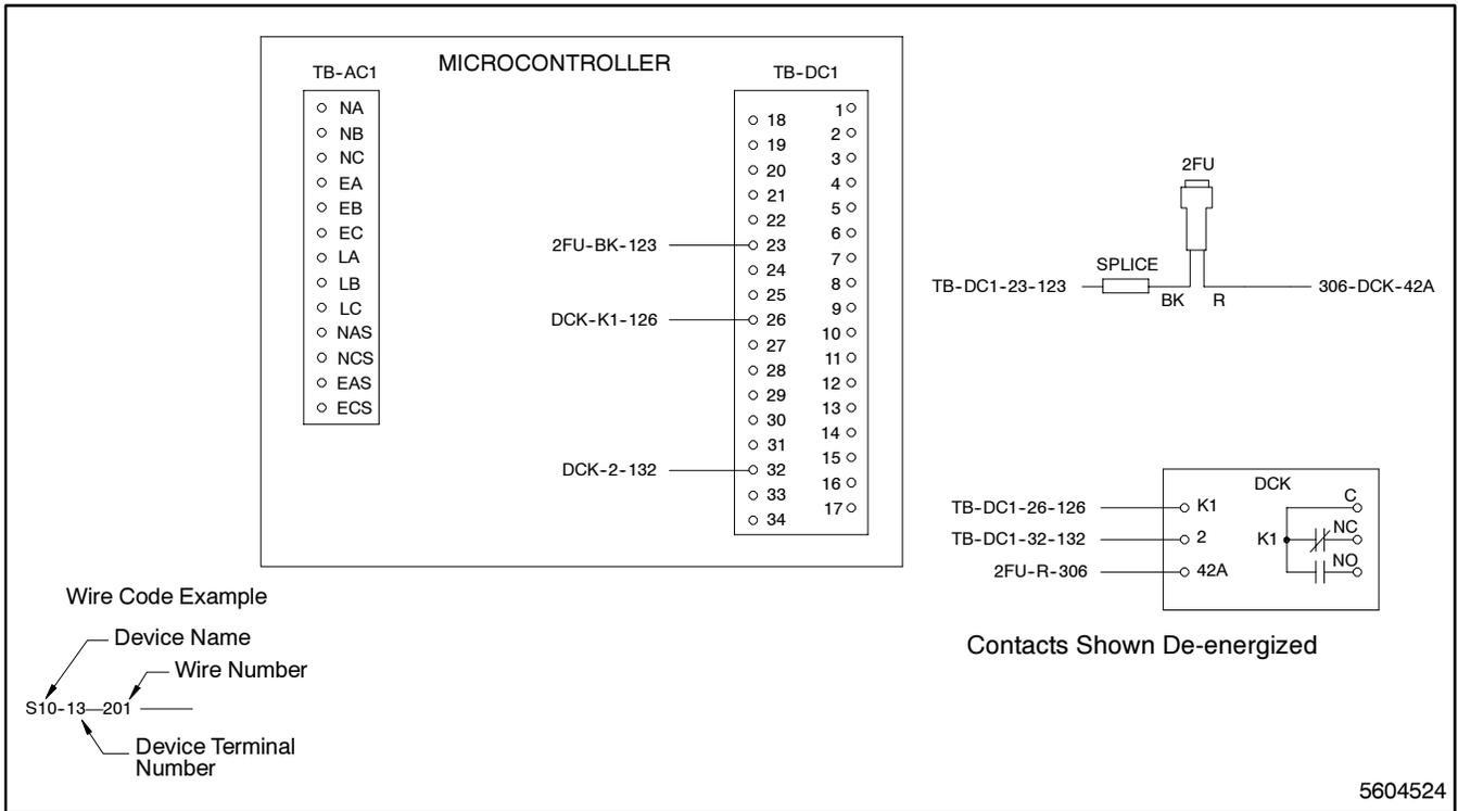
**Figure 5-19. Wiring Diagram—Option DD-14-K, Auxiliary Dry Contacts**
