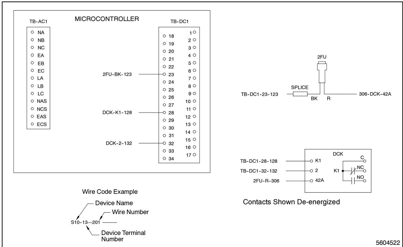
**Figure 5-17. Wiring Diagram—Option DD-14-H, Auxiliary Dry Contacts**
