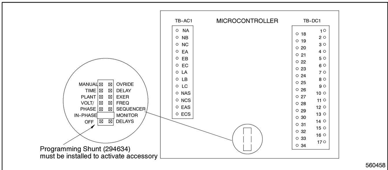
**Figure 4-19. Wiring Diagram—In-Phase Monitor, Option DD-34-A**
