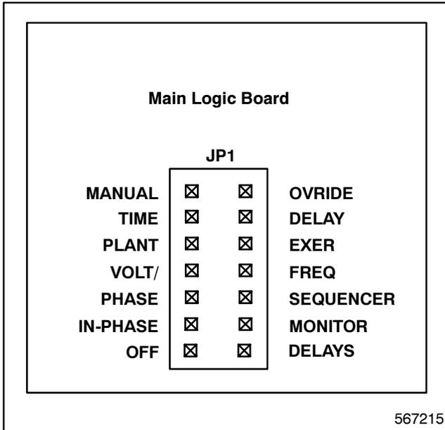
**Figure 1-5. MATS+ Logic Board Accessory Programming Shunts**
