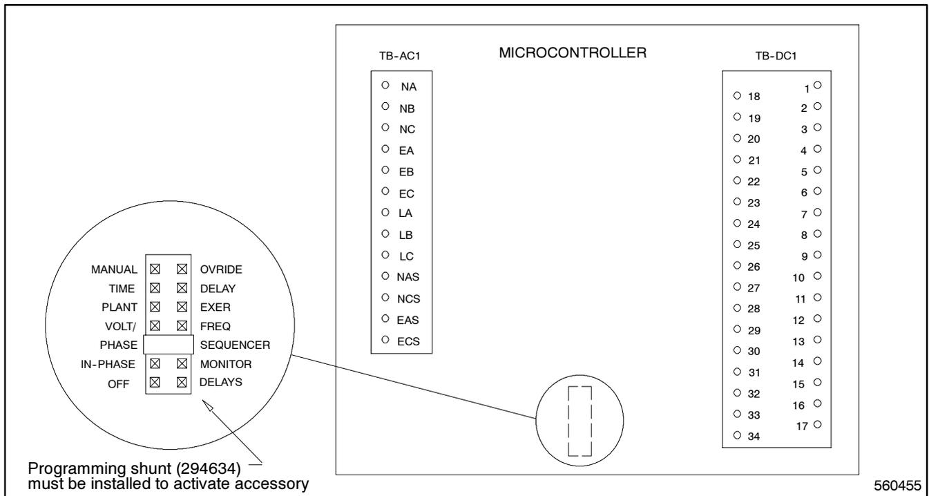
**Figure 4-21. Wiring Diagram—Source Monitor Phase Sequence, Option DD-34-Z**
