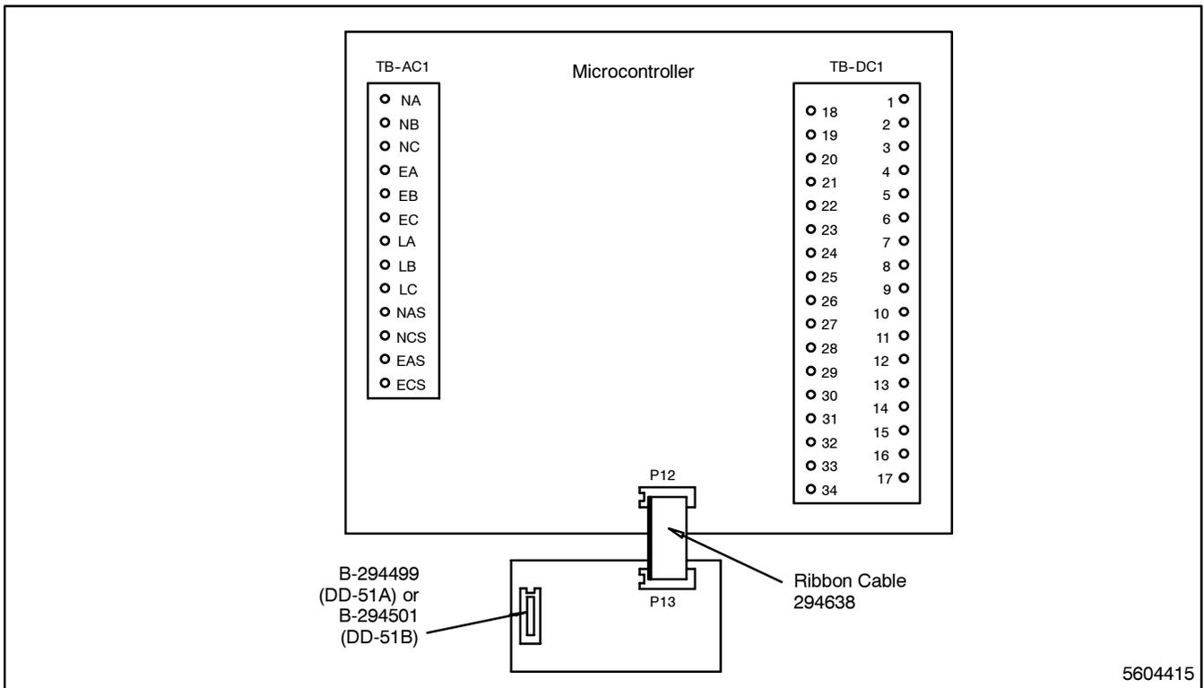
**Figure 5-73. Wiring Diagram—Option DD-51-A and DD-51-B, Remote Communications Board**
