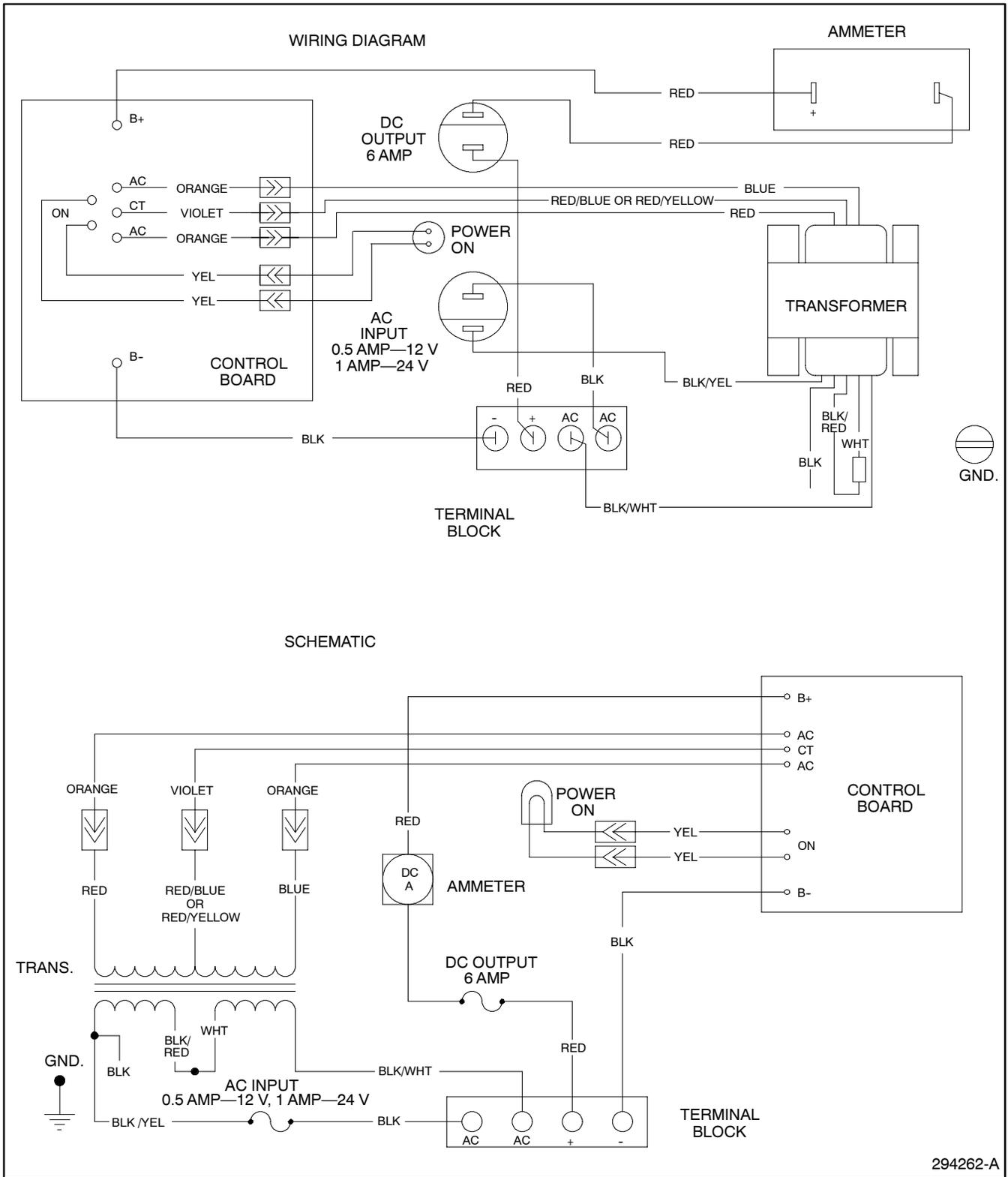
**Figure 5-56. Wiring Diagram—Option DD-24, Battery Charger 240-Volt Input**
