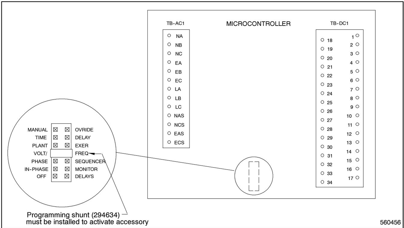
**Figure 4-22. Wiring Diagram—Voltage/Frequency Sensing, Option DD-34-J**
