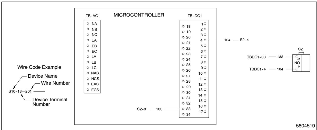
Figure 5-11. Wiring Diagram—Time Delay Override, Option DD-08-C
