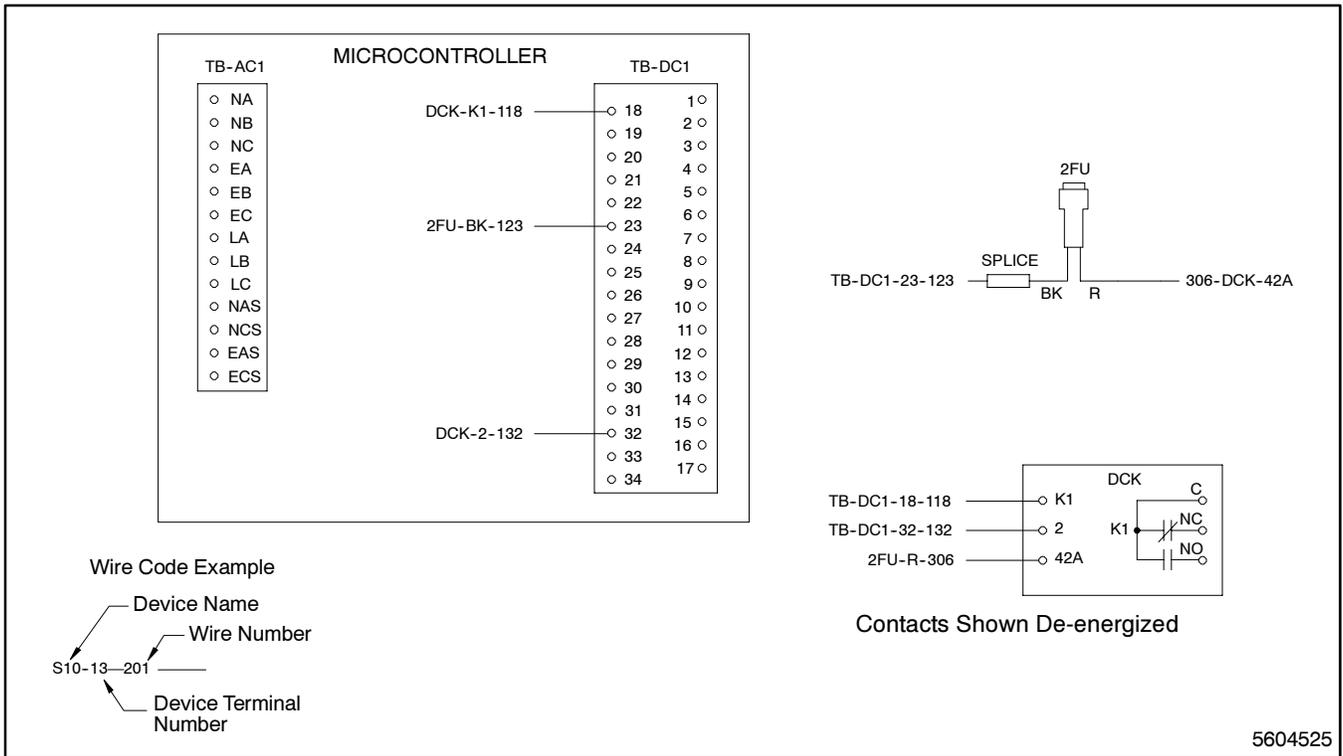
**Figure 5-20. Wiring Diagram—Option DD-14-L, Auxiliary Dry Contacts**
