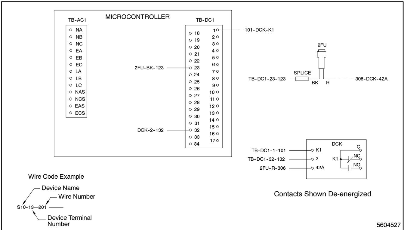
**Figure 5-22. Wiring Diagram—Option DD-14-N, Auxiliary Dry Contacts**
