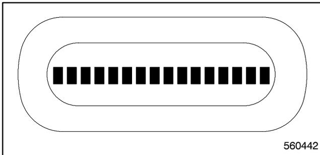
**Figure 4-2. The MATS+ LCD Display During a Lamp Test**
