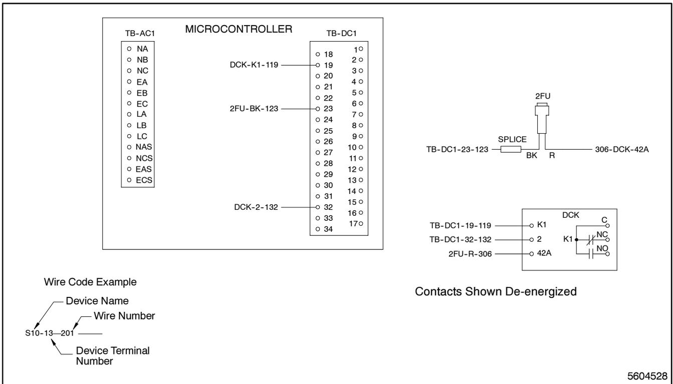
**Figure 5-23. Wiring Diagram—Option DD-14-P, Auxiliary Dry Contacts**
