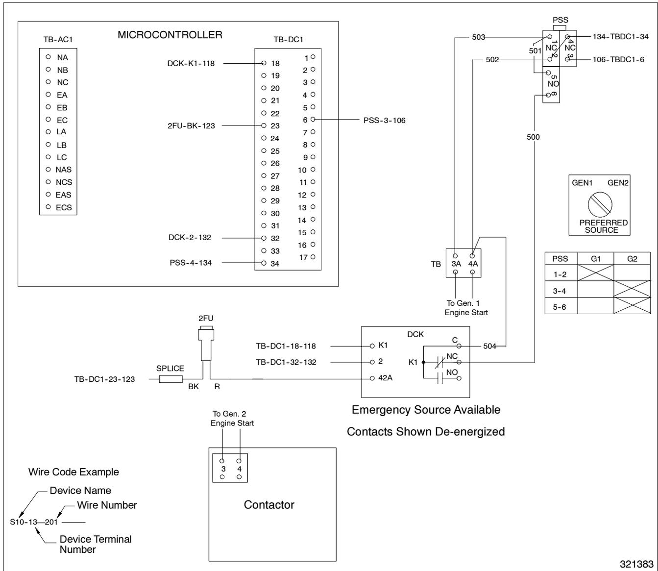
Figure 5-15. Wiring Diagram—Preferred Source Switch, Option DD-10-D
