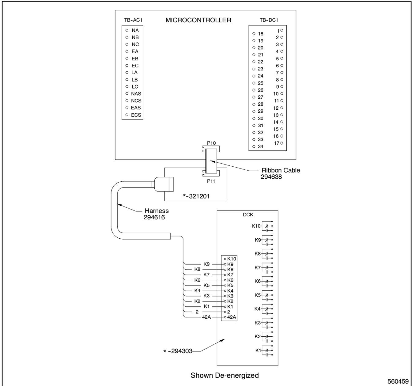
Figure 5-70. Wiring Diagram—Option DD-35-N, Load-Shedding Contacts
