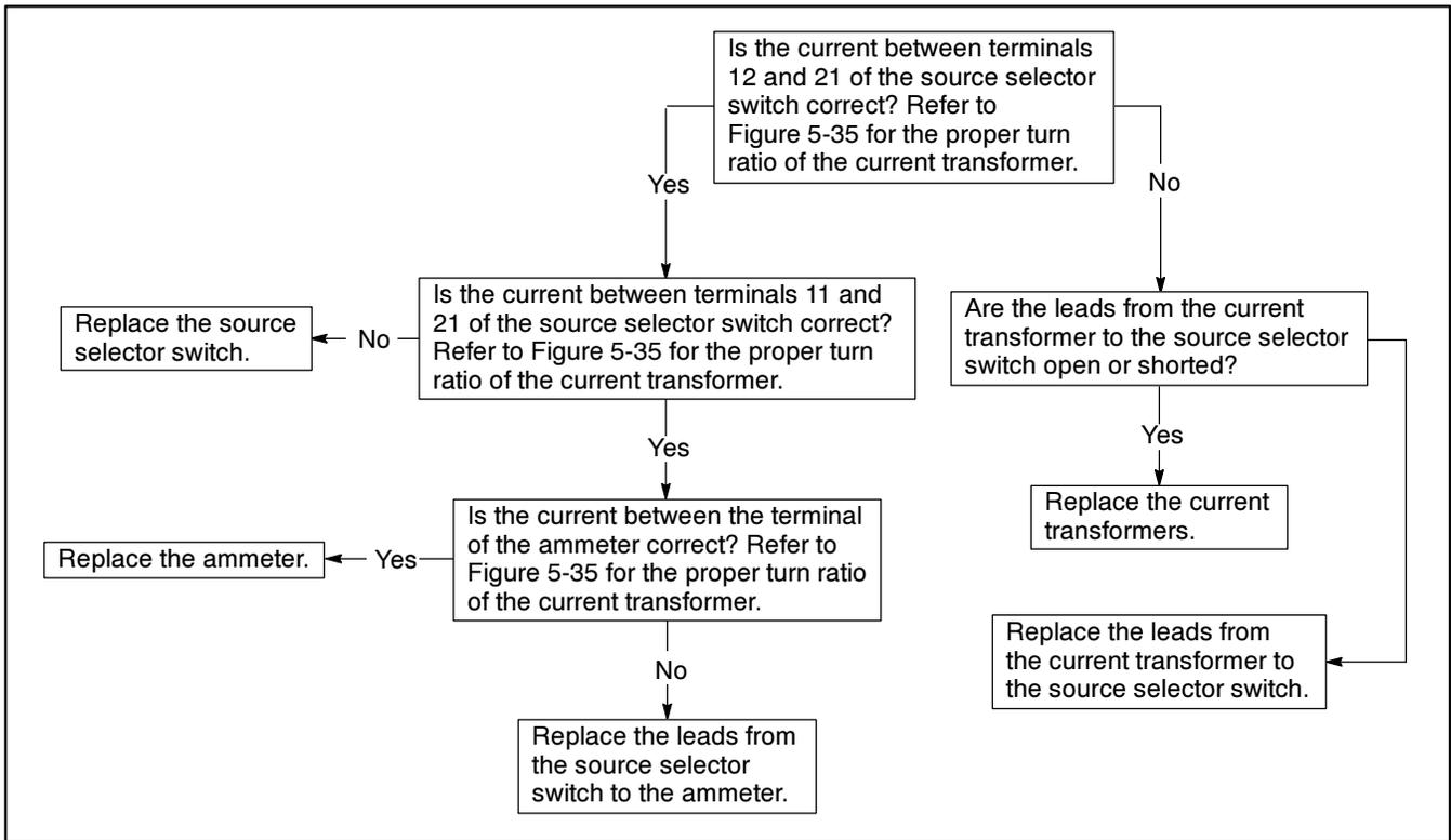
**Figure 5-37. Troubleshooting—Option DD-18-J, Ammeter Is Not Functioning**
