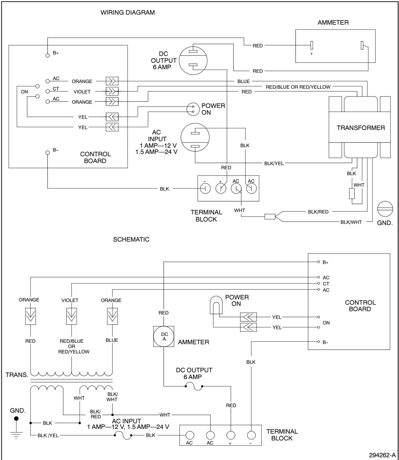
**Figure 5-54. Wiring Diagram—Option DD-24, Battery Charger 120-Volt Input**
