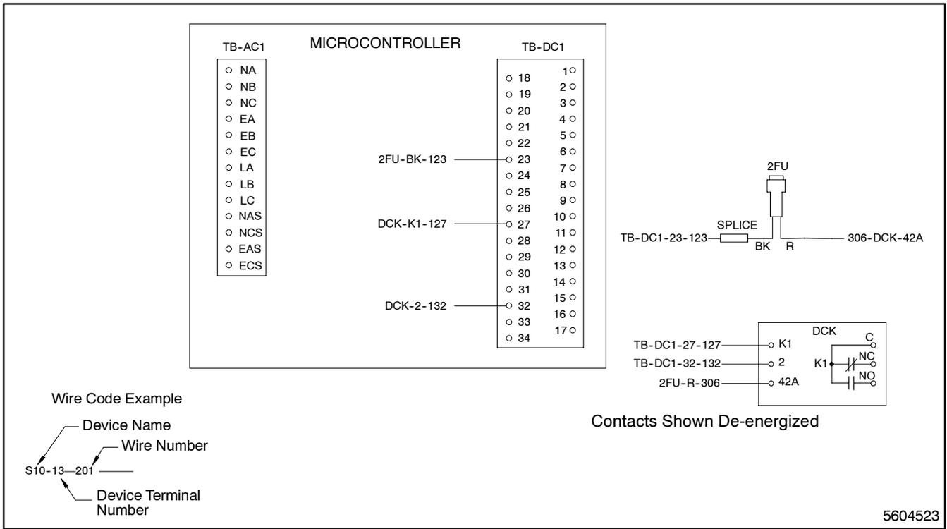
**Figure 5-18. Wiring Diagram—Option DD-14-J, Auxiliary Dry Contacts**
