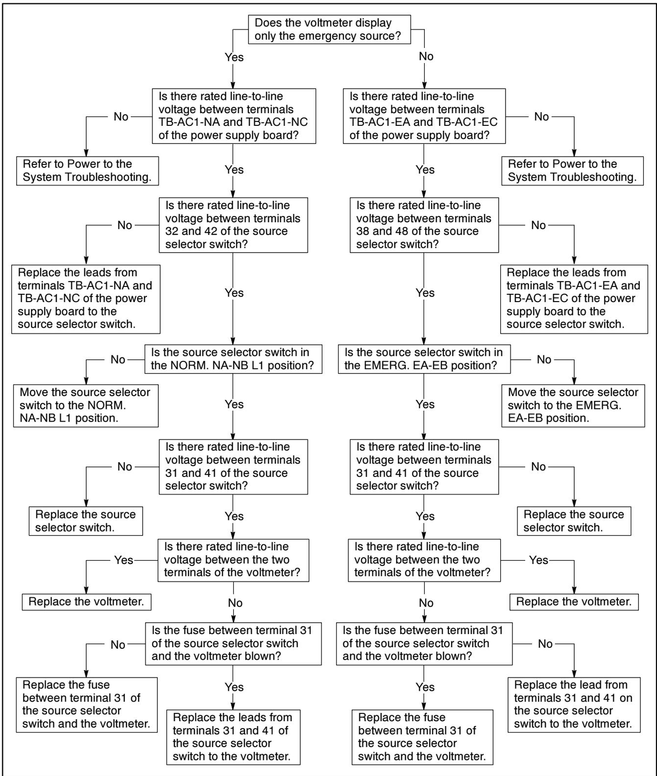
**Figure 5-38. Troubleshooting—Option DD-18-J, Voltmeter Is Not Functioning**
