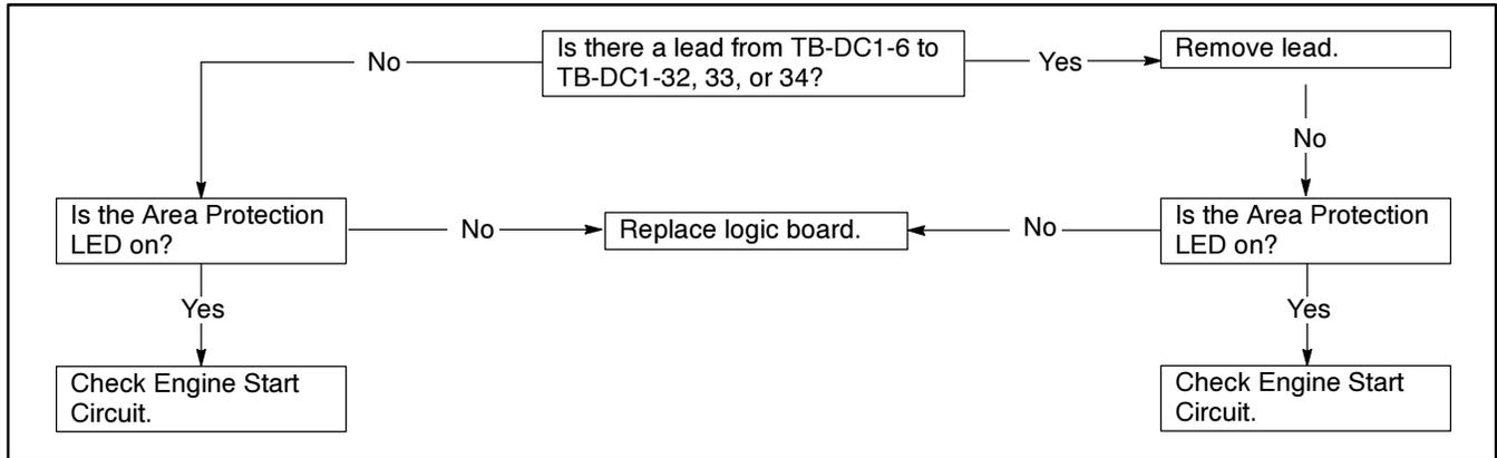
Figure 4-13. Troubleshooting—Area Protection Does Not Turn On
