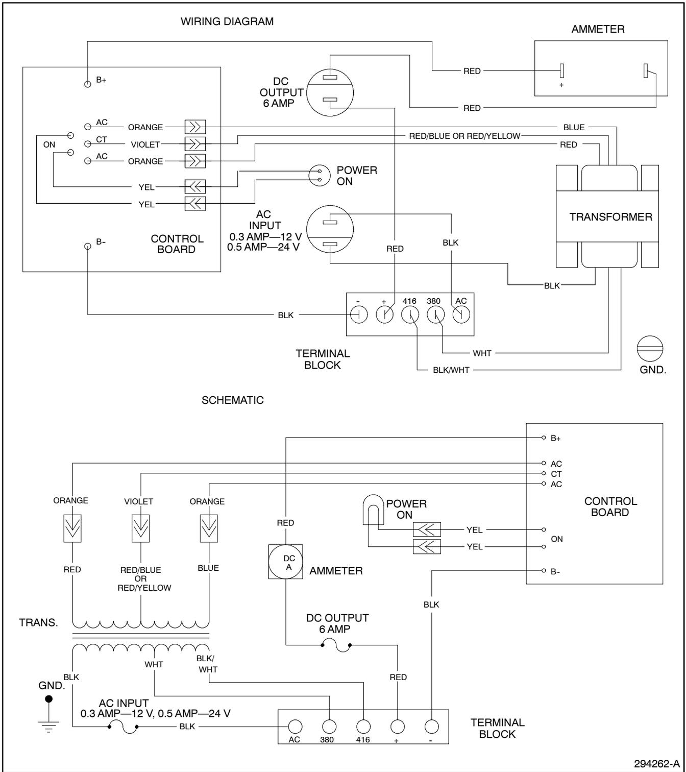
**Figure 5-57. Wiring Diagram—Option DD-24, Battery Charger 380/416-Volt Input**
