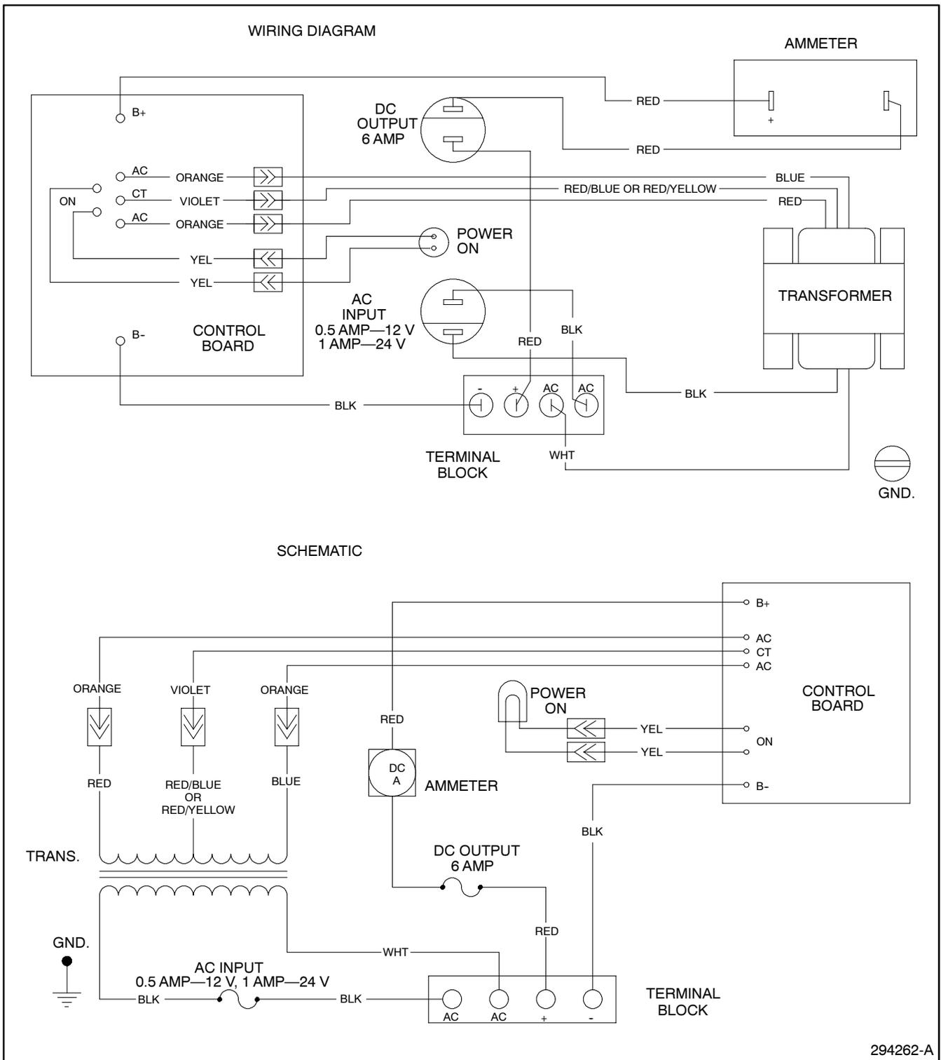
**Figure 5-55. Wiring Diagram—Option DD-24, Battery Charger 220-Volt Input**
