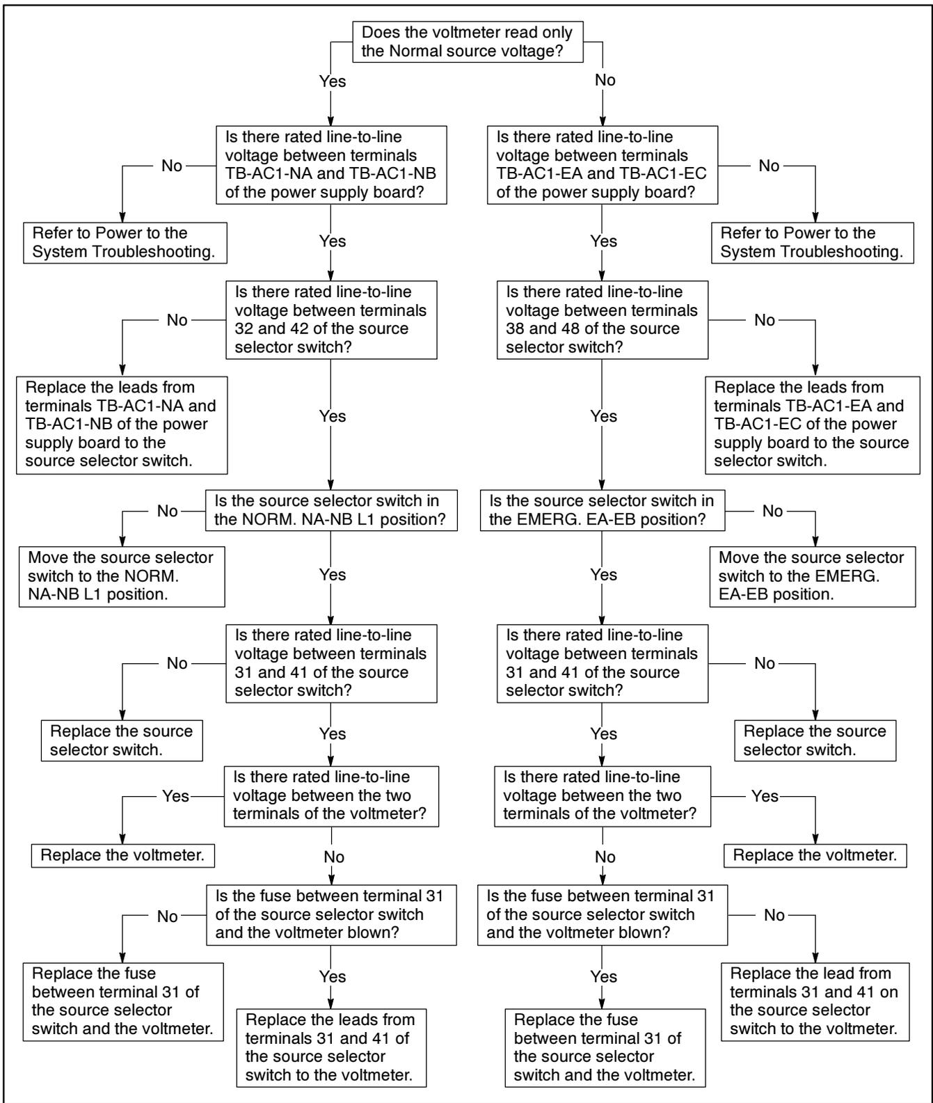
**Figure 5-36. Troubleshooting—Option DD-18-J, Voltmeter Is Not Functioning**
