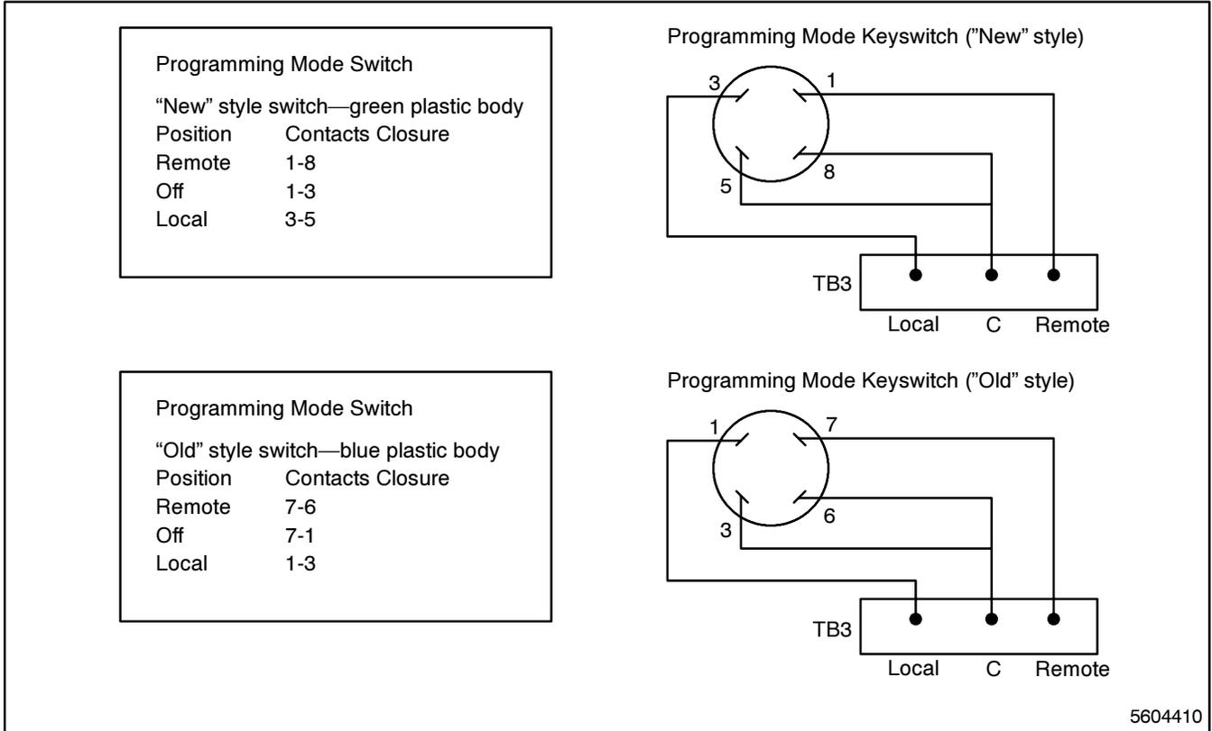
**Figure 4-10. Wiring Diagram—Programming Mode Keyswitch**
