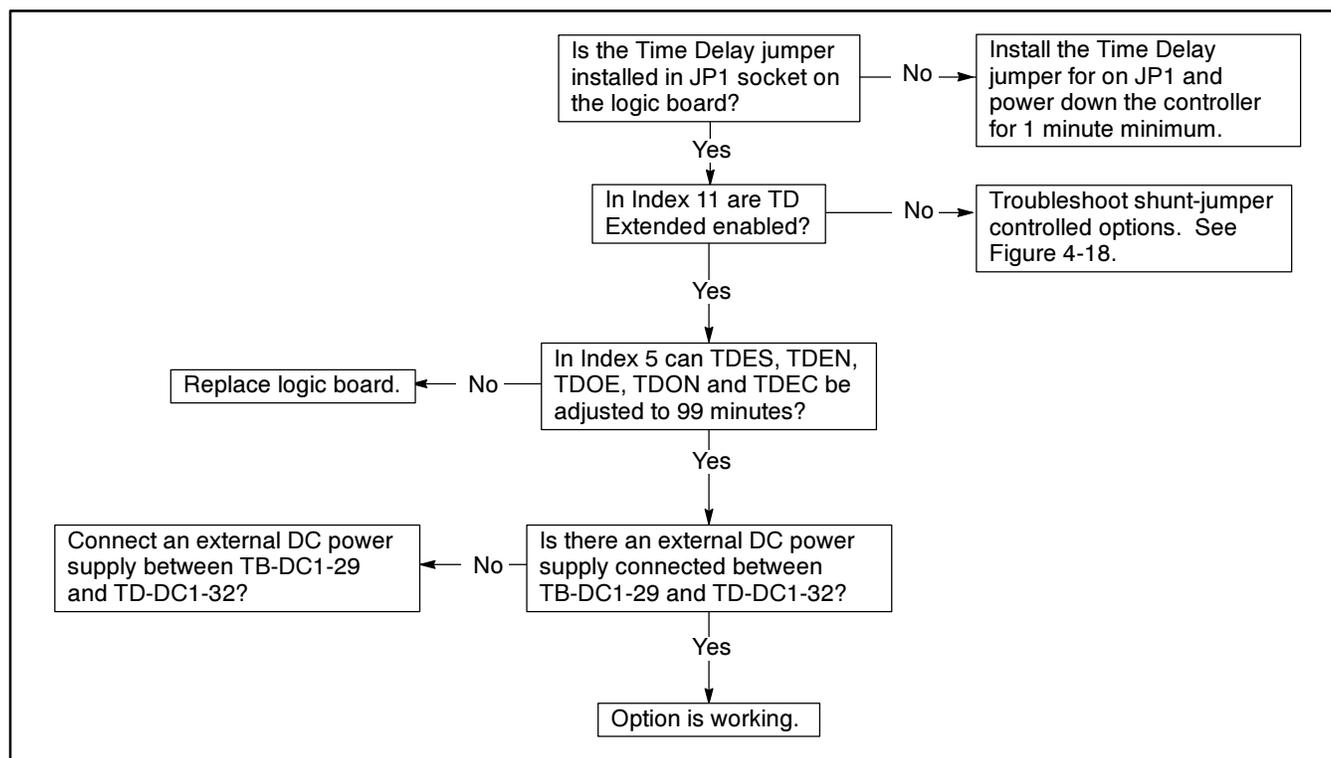
**Figure 4-31. Troubleshooting—Extended Time Delays Do Not Work**
