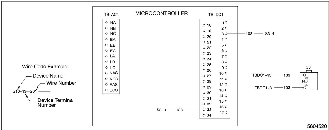
Figure 5-13. Wiring Diagram—Time Delay Override, Option DD-08-D
