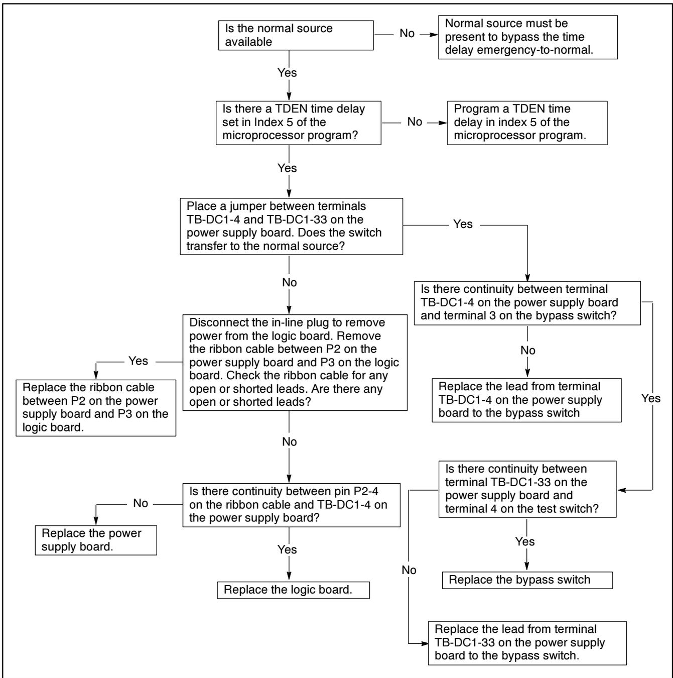
**Figure 5-12. Troubleshooting—Option DD-08-C, Emergency-to-Normal Time Delay Pushbutton Does Not Work**
