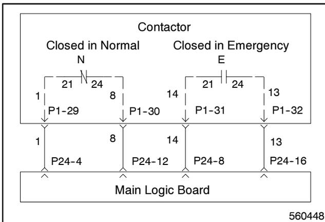
Figure 4-8. Wiring Diagram—Contactor Position Auxiliary Switches
