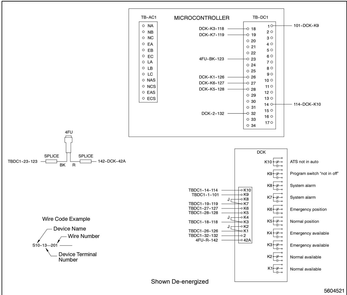
Figure 5-16. Wiring Diagram—Option DD-14-G, Auxiliary Dry Contacts
