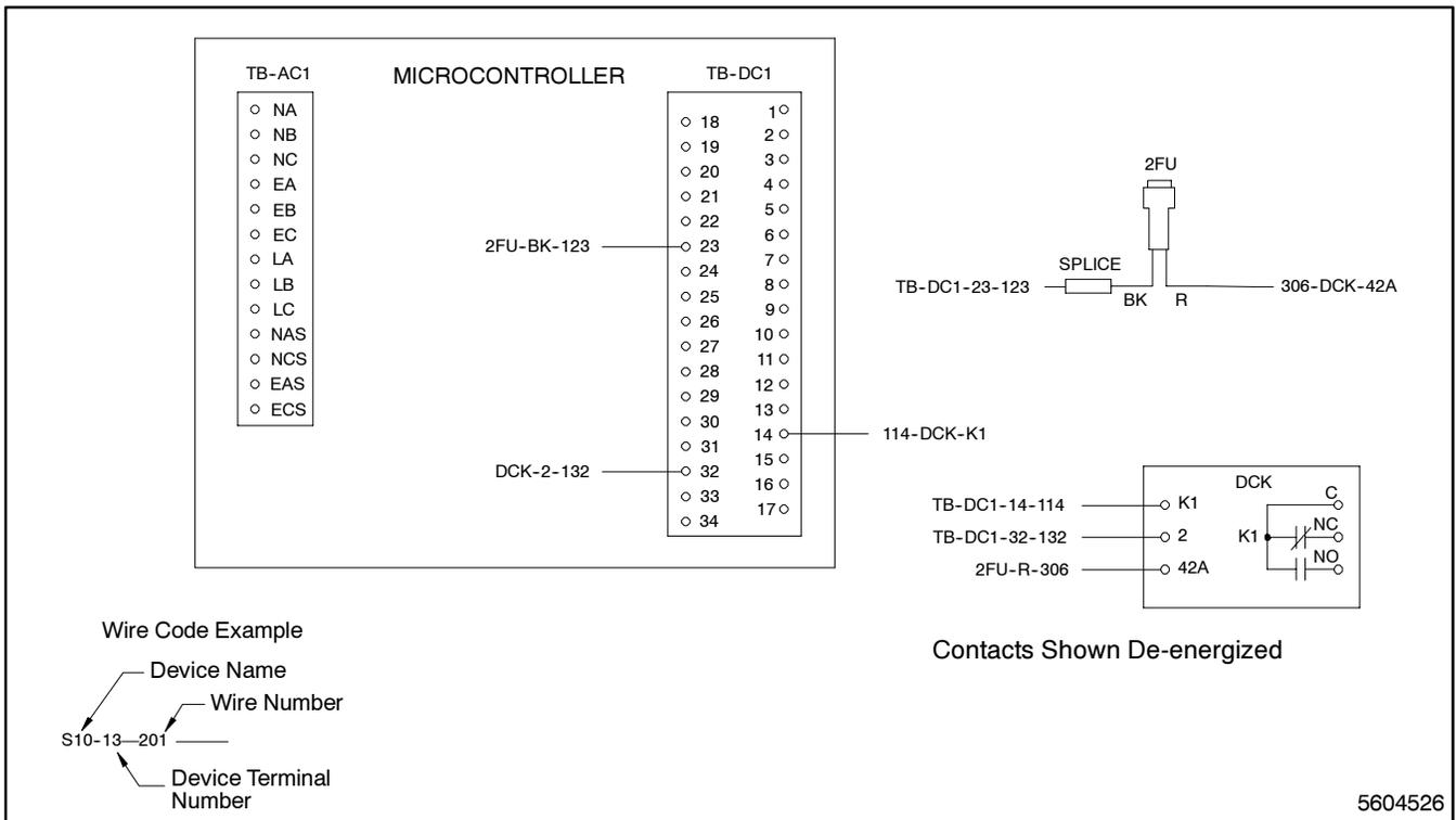
**Figure 5-21. Wiring Diagram—Option DD-14-M, Auxiliary Dry Contacts**
