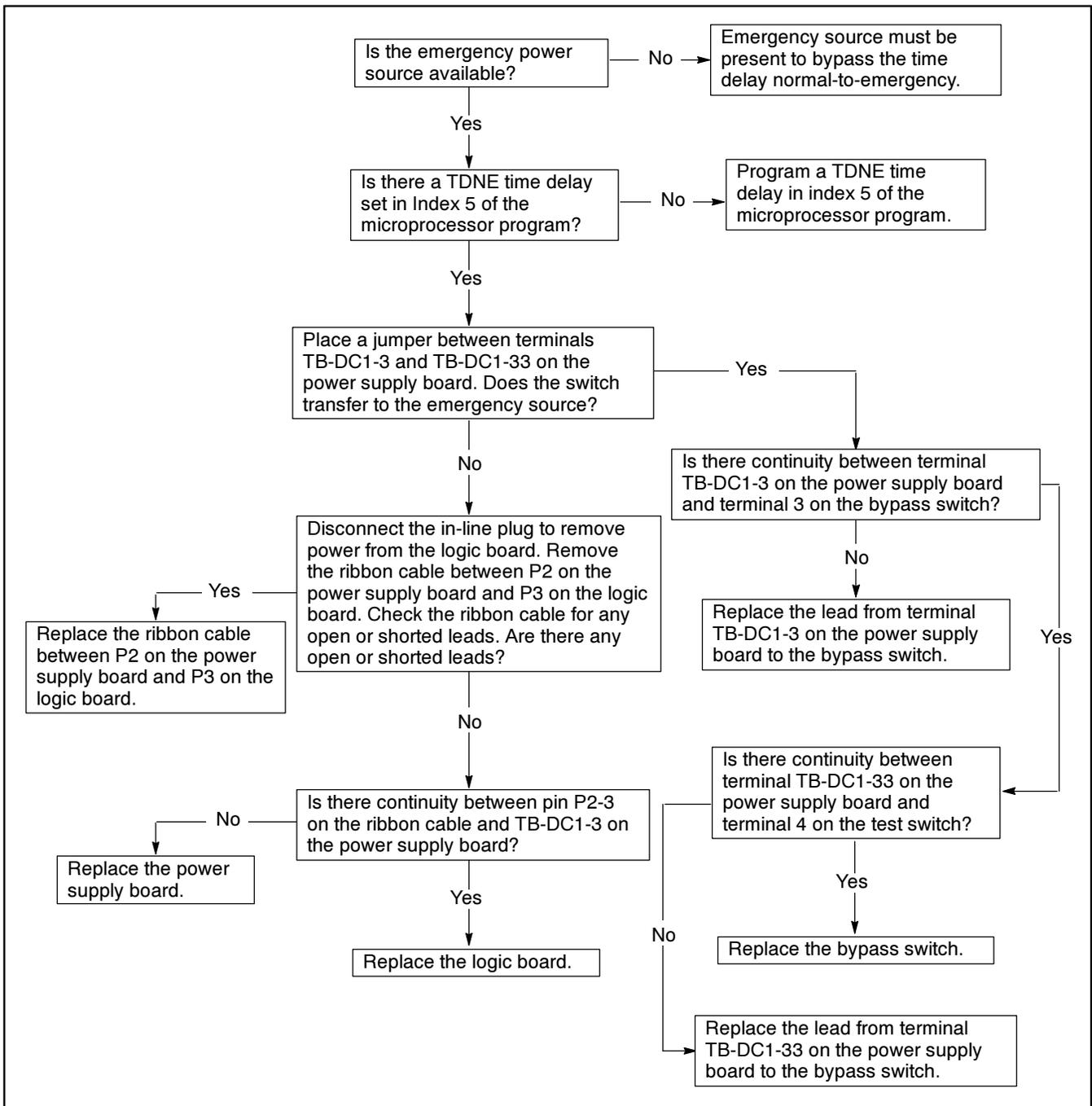
**Figure 5-14. Troubleshooting—Option DD-08-D, Normal-to-Emergency Time Delay Pushbutton Does Not Work**
