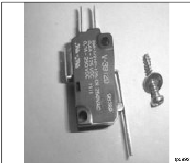
Figure 6-11 Microswitch and Mounting Screw
