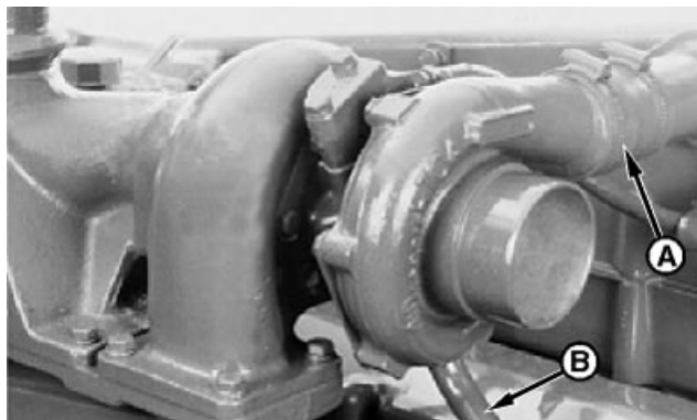
A—Crossover Tube B—Oil Return Line
