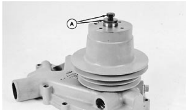
A—Cap Screw and Washer
