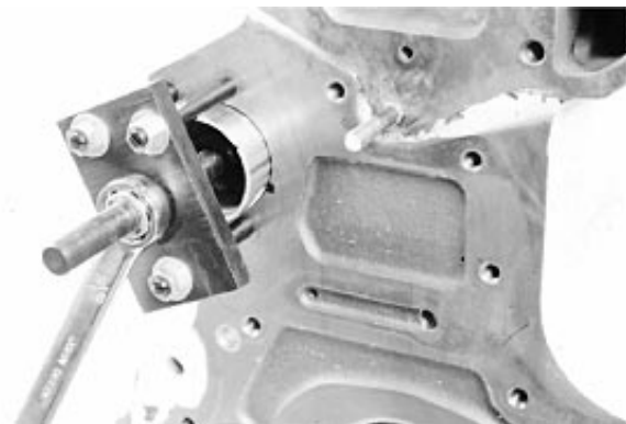
A—Threaded Spacers B—Forcing Plate C—Bushing Puller
