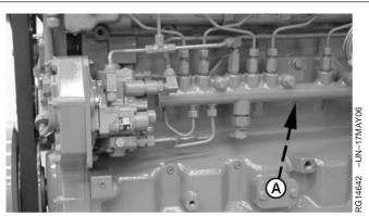
Engine Block Coolant Drain Plug
