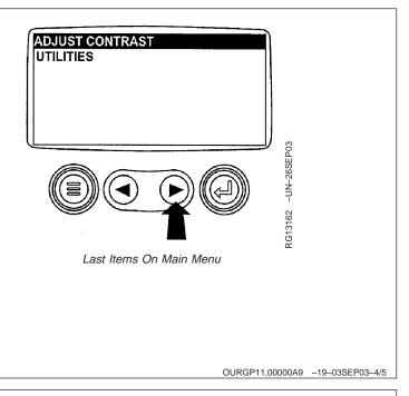
5. Use the arrow keys to scroll to the desired menu item or press the "Menu Button" to exit the main menu and return to the engine parameter display.
