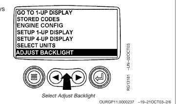
3. Once the "Adjust Backlight" menu item has been GO TO 1-UP DISPLAY highlighted, press the "Enter" key to activate the STORED CODES "Adjust Backlight" function. ENGINE CONFIG SETUP 1-UP DISPLAY SETUP 4-UP DISPLAY SELECT UNITS RG13182 -UN-02OCT03 ADJUST BACKLIGHT Press Enter Key OURGP11,0000237 -19-21OCT03-3/6 4. Use the "Arrow" keys to select the desired backlight ADJUST BACKLIGHT intensity. RG13183 -UN-29SEP03 Adjust Backlight Intensity Continued on next page OURGP11,0000237 -19-21OCT03-4/6
