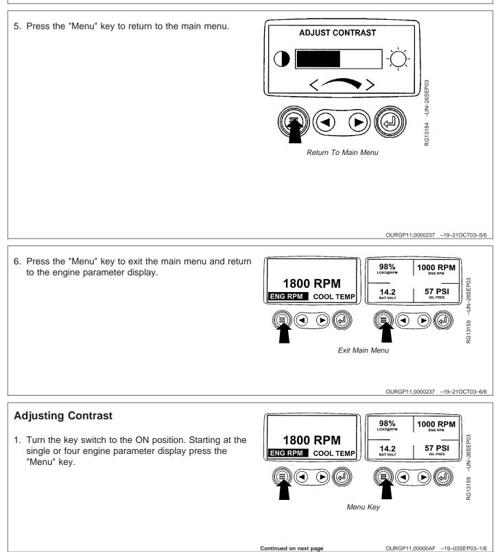
2. The main menu will be displayed. Use the "Arrow" keys to scroll through the menu until "Adjust Contrast" is highlighted.
