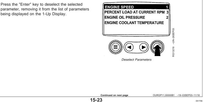
12. Use the "Arrow" keys to scroll and highlight the desired parameter that has not been selected for display (parameter without a number to right of it).
