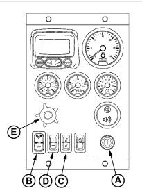
Start And Idle Engine Controls On Panel
