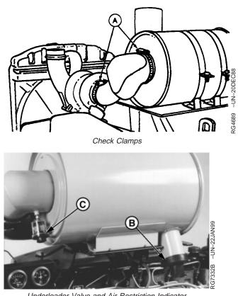
Underloader Valve and Air Restriction Indicator
