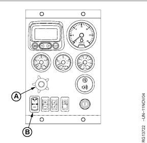
Analog Throttle Control and Speed Select Switch On Panel
