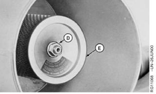
Retaining Nut and Secondary Element
