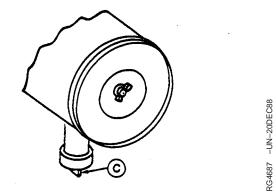
Dust Unloader Valve and Restriction Indicator
