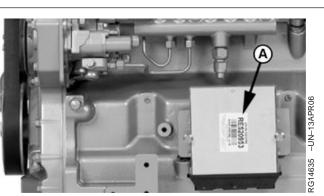
Record Engine Control Unit (ECU) Serial Number
