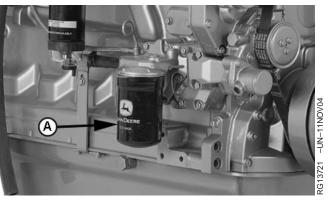
Oil Filter And Mounting Header
