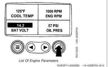
9. The parameter that is highlighted is the selected parameter for the screen. Use the "arrow" keys to highlight the new parameter to be placed in the "4-Up Display".
