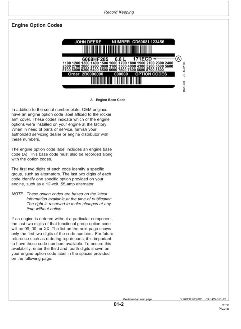
NOTE: Your engine option code label may not contain all option codes if an option has been added after the engine left the producing factory.
