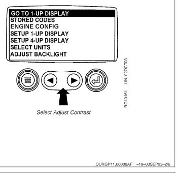
3. Once the "Adjust Contrast" menu item has been STORED CODES highlighted, press the "Enter" key to activate the **ENGINE CONFIG** "Adjust Contrast" function. SETUP 1-UP DISPLAY SETUP 4-UP DISPLAY SELECT UNITS ADJUST BACKLIGHT RG13185 -UN-02OCT03 ADJUST CONTRAST Press Enter Key OURGP11,00000AF -19-03SEP03-3/6 4. Use the "Arrow" keys to select the desired contrast ADJUST CONTRAST intensity. RG13186 -UN-29SEP03 Adjust Contrast Intensity Continued on next page OURGP11,00000AF -19-03SEP03-4/6
