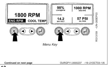
2. The main menu will be displayed. Use the "Arrow" keys to scroll through the menu until "Adjust Backlight" is highlighted.
