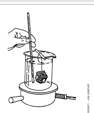
Testing Thermostat Opening Temperature
