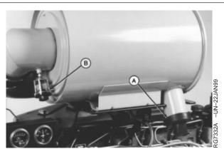
Dust Unloader Valve and Indicator Gauge
