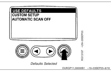
7. The display parameters are reset to the factory defaults, then the display will return to the "Setup 1-Up Display" menu.
