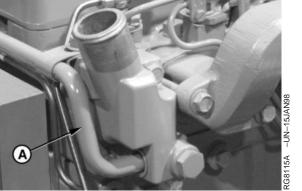
Thermostat Cover-to-Coolant Pump Tube DPSG,RG34710,112 -19-23NOV01-1/5
