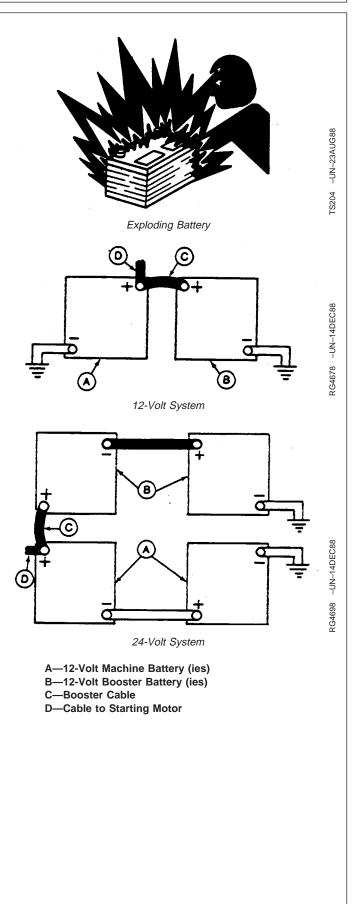
Start the engine. Disconnect jumper cables immediately after engine starts. Disconnect NEGATIVE (–) cable first.
