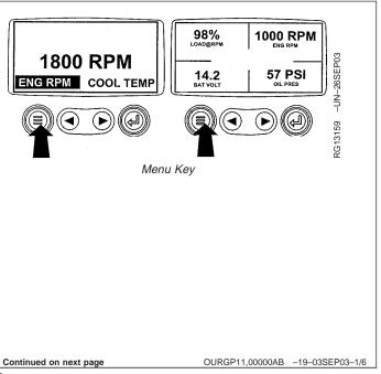
2. The main menu will be displayed. Use the "Arrow" keys to scroll through the menu until "Engine Config" is highlighted.
