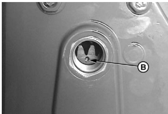
High pressure pump gear timing mark
