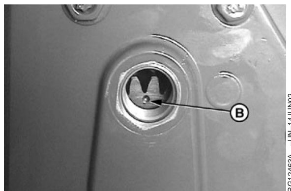
High pressure pump gear timing mark
