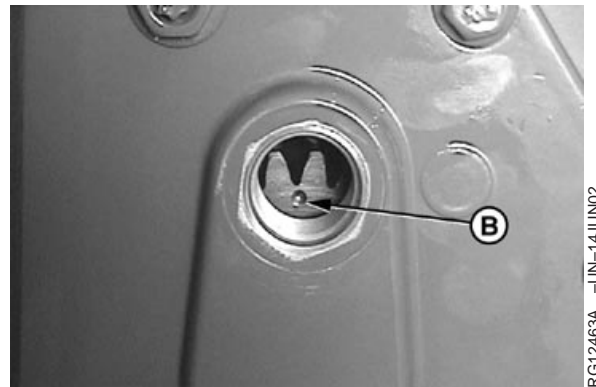
High pressure pump gear timing mark
