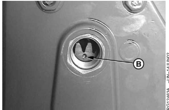
High pressure pump gear timing mark
