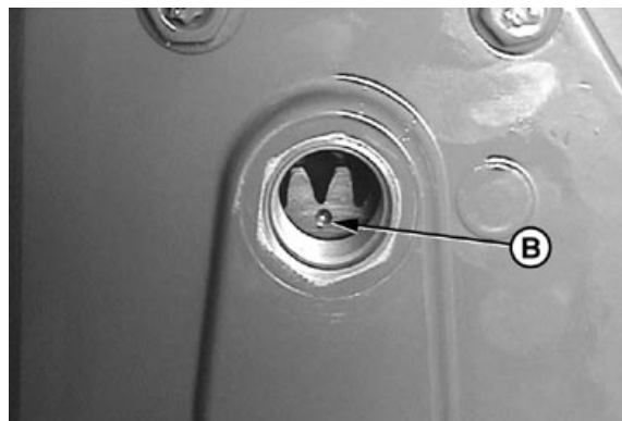
High pressure pump gear timing mark
