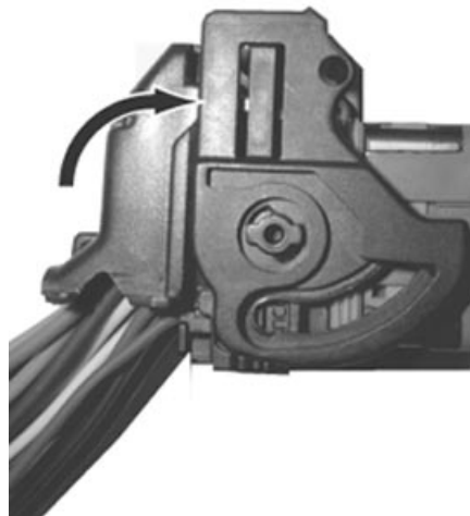
Rotate lock 90 Degrees
