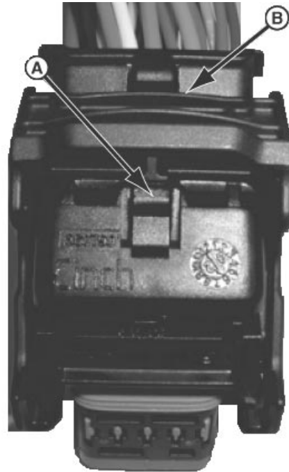
Tab and Connector Lock
