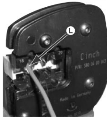
Wire Onto Terminal in Crimping Pliers
