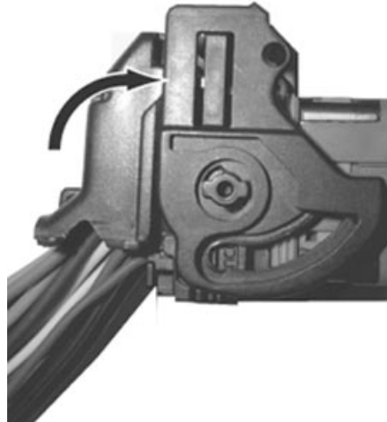
Rotate lock 90 Degrees
